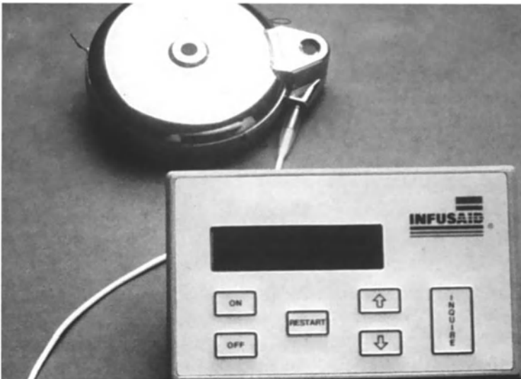
Fig. 5. The InfusaID programmable pump and portable programmer
