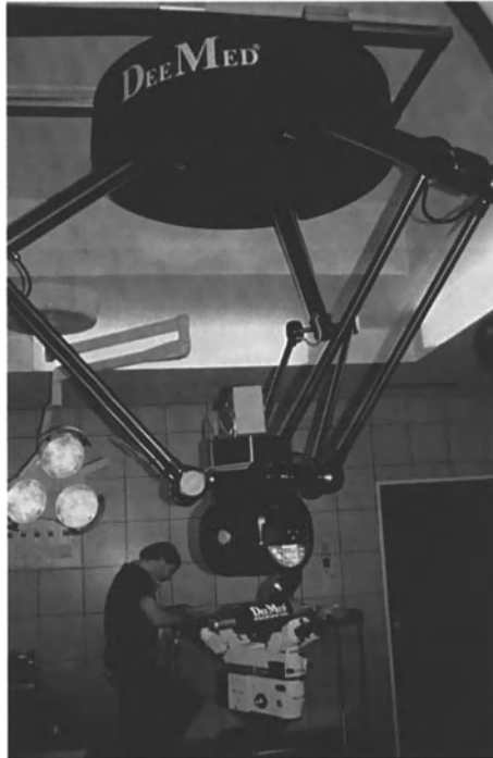
Fig. 11. The G.P.R. robot microscope holder
