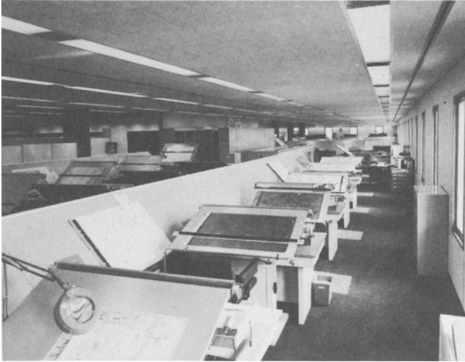
Figure 1.22 Office with parallel motion equipment (Courtesy of the Elite Manufacturing Co. Ltd)
