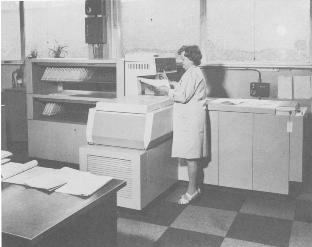
Figure 2.9 High-speed printer with automatic document feed and collation (courtesy of the London Borough of Ealing)
