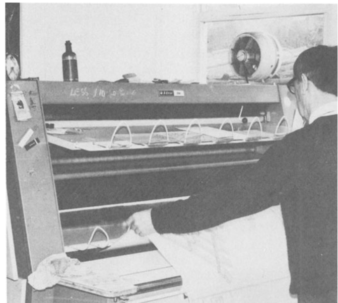
Figure 2.5 Dry or ammonia process.
