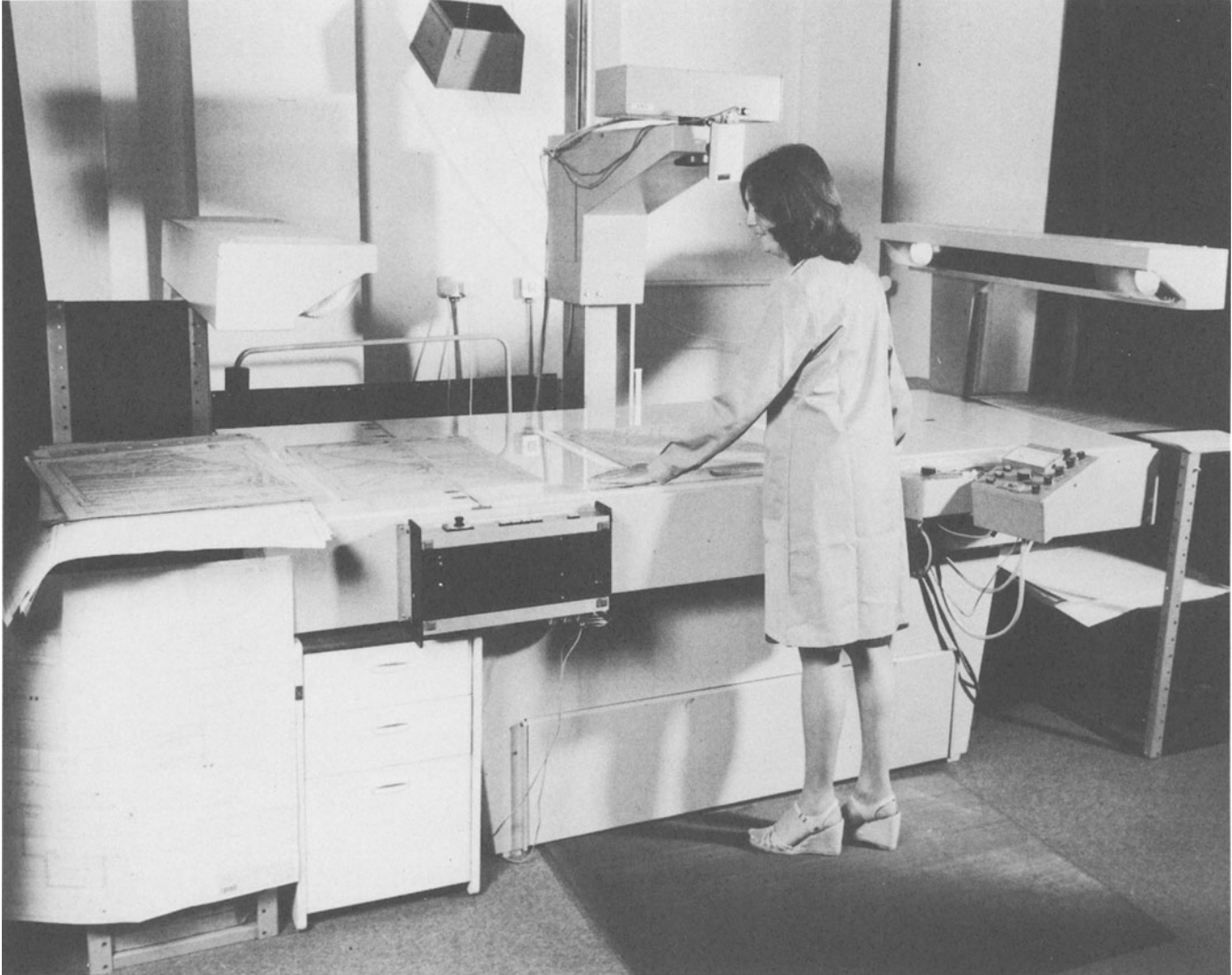
Figure 2.10 35 mm microfilm camera with electronic exposure metering and enlarging facilities (courtesy of the London Borough of Ealing)
