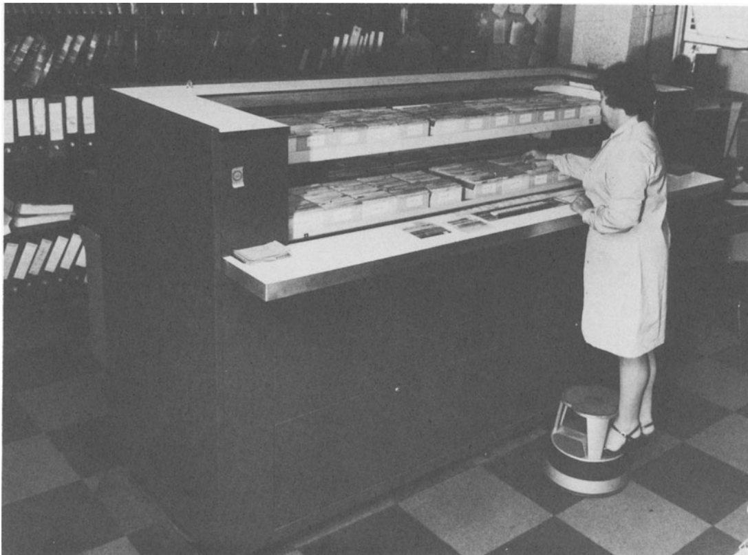
Figure 2.6 Automated microfilm filing and retrieval unit (courtesy of the London Borough of Ealing)
