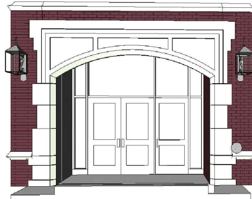
Stone trimmed opening created as an in-place family to interface with project conditions.
