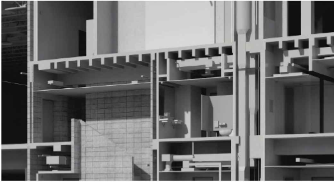
Revit model of an existing building, with architecture, structural, mechanical, plumbing and electrical all modeled.
