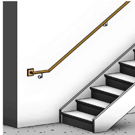
FIGURE 5-4.32 Handrail only with supports at 6'-0" O.C. max.
