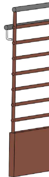
FIGURE 5-4.12 Railing with stringer
