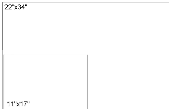
FIGURE 14-1.17 Standard sheet size of 22"x34" can be printed to 11"x17" at half scale
