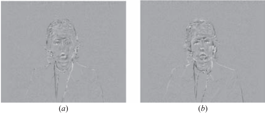
Figure 7.11 Motion-compensated prediction error (a) with and (b) without half-pixel precision
