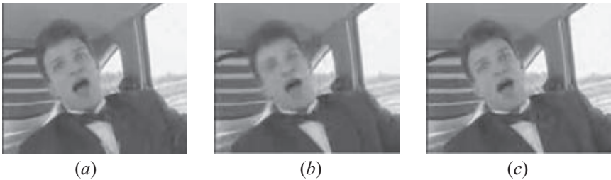
Figure 10.34 A snap shot of Carphone coded at 40 kbit/s, 10 Hz, (a) H.263, (b) SNR-scalable H.263 and (c) wavelet SPIHT
