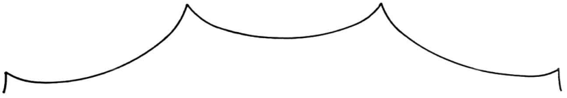
54. Section of the Doric column displaying outline of fluting (Pikionis 1935).
