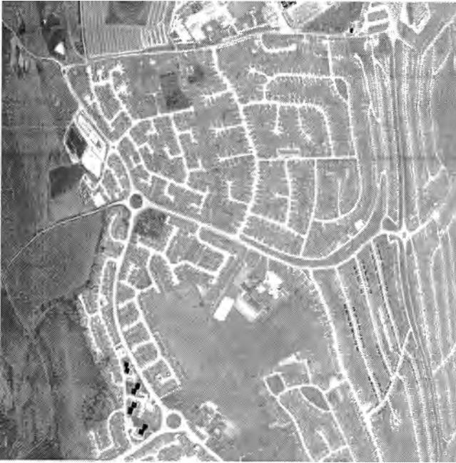
Fig. 3.1. The image used in all examples in this paper. It is a infra-red line scan image taken from 3000ft by an aircraft, 512 \times 512 pixels, 8 bits per pixel.
