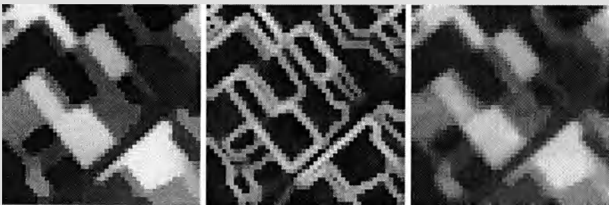
Fig. 3.2. Processed SPOT-image and its edge map (left and middle) and the result of a 3 \times 3 median filtering (right).
