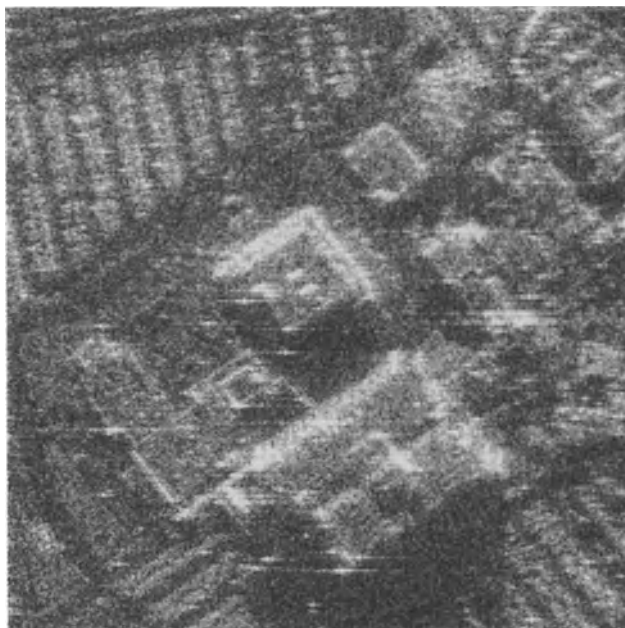
Figure 4.9 Urban SAR scene degraded by a rapidly varying (high frequency) phase error. The peak-to-peak phase variation corresponds to only 1/4 wavelength of relative range error.
