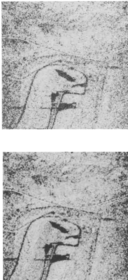
Figure 5.15 A comparison of two correlation window sizes for the landfill interferometric change-detection images. The upper image was correlated using 3x3 windows. The lower image used 7x7 correlation windows. The larger sample size (the 7x7 windows) gives a much better estimate of the true values of \alpha .
