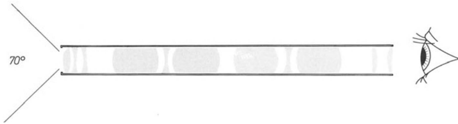
Fig. 2. The Hopkins solid rod lens system which makes greater use of the internal diameter of the containing tube and which avoids problems of the alignment of lenses and the use of spacer tubes
