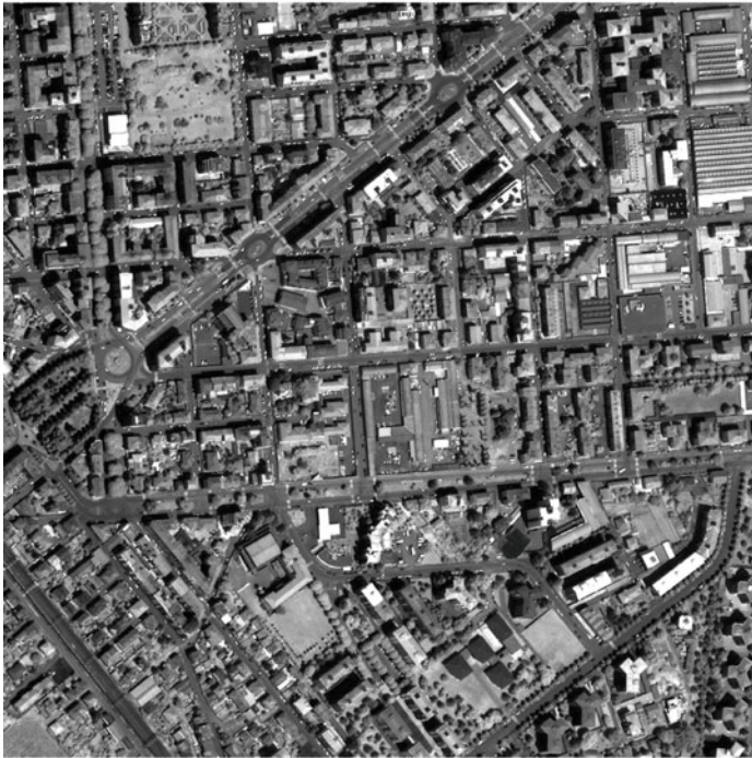
Fig. 1.5 Portion of an IKONOS image collected over Alessandria, Italy: a panchromatic channel at 1-m spatial resolution; b color composite of the red , green , and blue multispectral channels at 4-m spatial resolution
