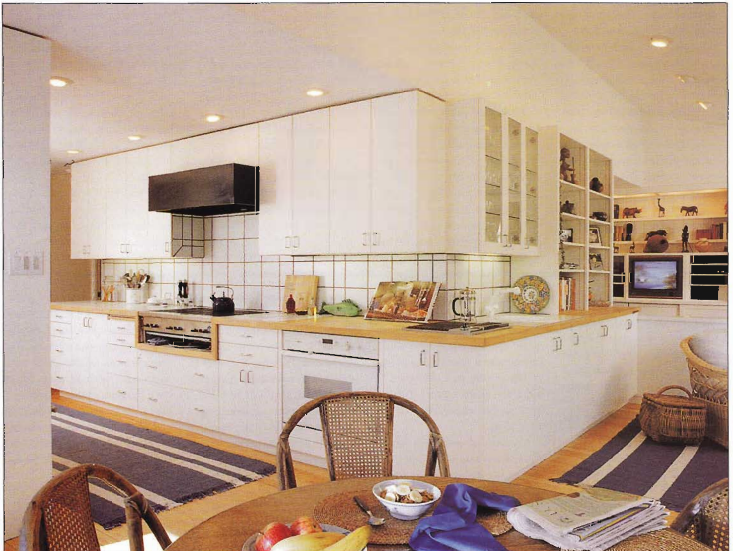
One of the primary work centers of every kitchen is dedicated to cooking. Here, a component system is made up of a separate cooktop with storage beneath, an under-counter oven, and a grill. Plan flame-resistant surface treatments, such as this white ceramic tile, on either side of each cooking appliance to use for setting down hot foods.
