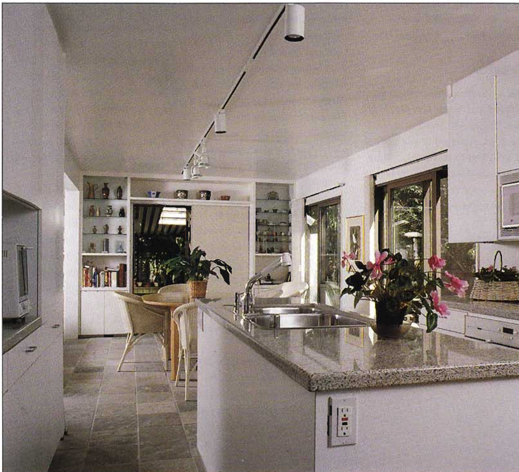
Consider combining several types of lighting within your kitchen. Here, tracks illuminate the work centers while small recessed lights spotlight items on the display shelves.
