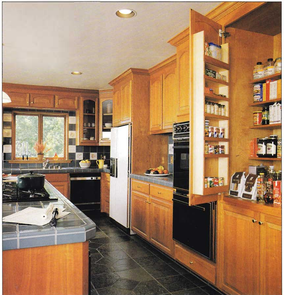
If your wish list includes a pantry but your floor plan doesn't allow space for one, consider a tall pantry cabinet equipped with door shelves, which handles dry storage needs in a minimum of space.
