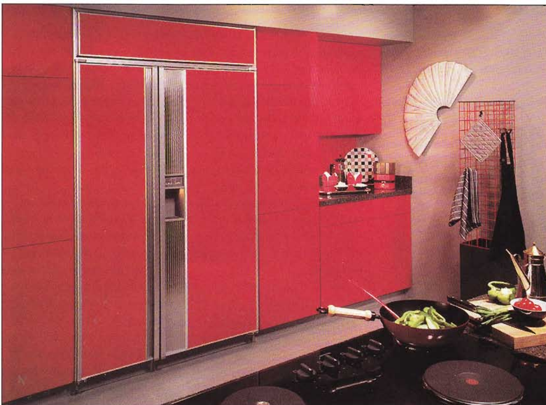
Plan landing space within the refrigerator center to set groceries while putting them away. The ideal landing is a minimum of 15 inches wide on the latch side of the refrigerator; it can also be located across from the appliance. The landing for this subzero refrigerator doubles as a food-preparation surface next to the cooktop.
