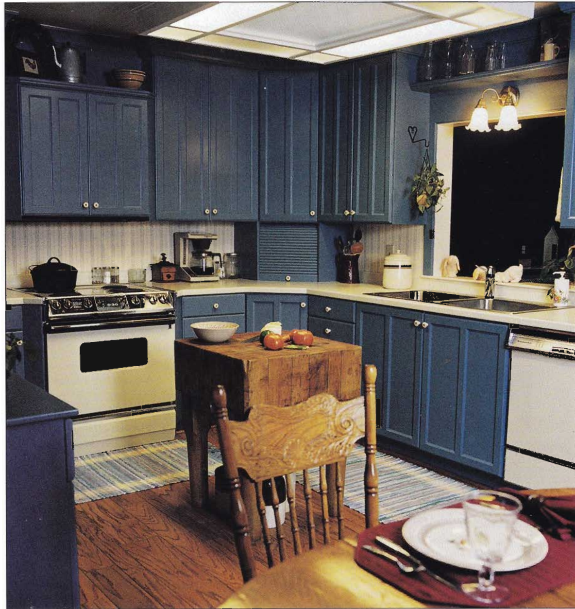
When well designed, manufactured materials can be effective in even a traditional kitchen with a country theme. Here a double-bowl stainless steel sink has a self-rim mount that has been installed over a solid-surface-material countertop.
