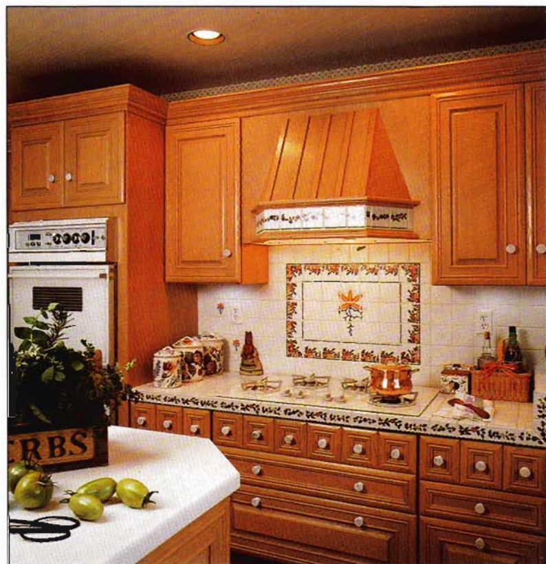
Individual burners can be aligned in different ways to best serve your needs. Four in-line and four in a square are the most common configurations. Here the back burners are offset from the front ones, which allows for large pots to be used without them overlapping the burners.
