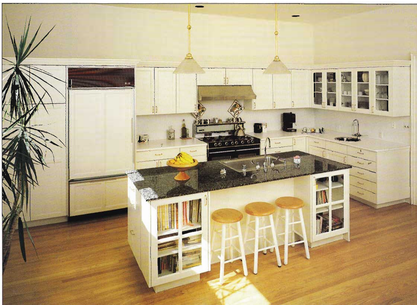
Check local codes before choosing sink accessories. Some codes disallow a hose sprayer, for example, in order to save water. Others require dishwasher air gaps—seen here on the deck of the island sink—for sanitary efficiency.
