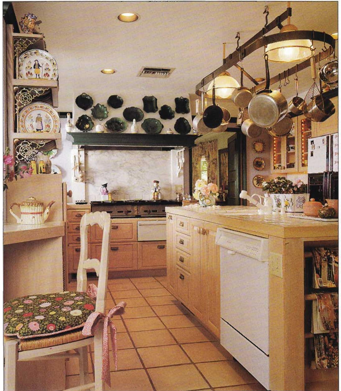
When planning a dishwasher located within an island cleanup center, be sure to incorporate power needs, including a convenient location for the on-off switch, and to account for enough aisle room for traffic even when the dishwasher door is open. Another view of this kitchen appears on page 29.
