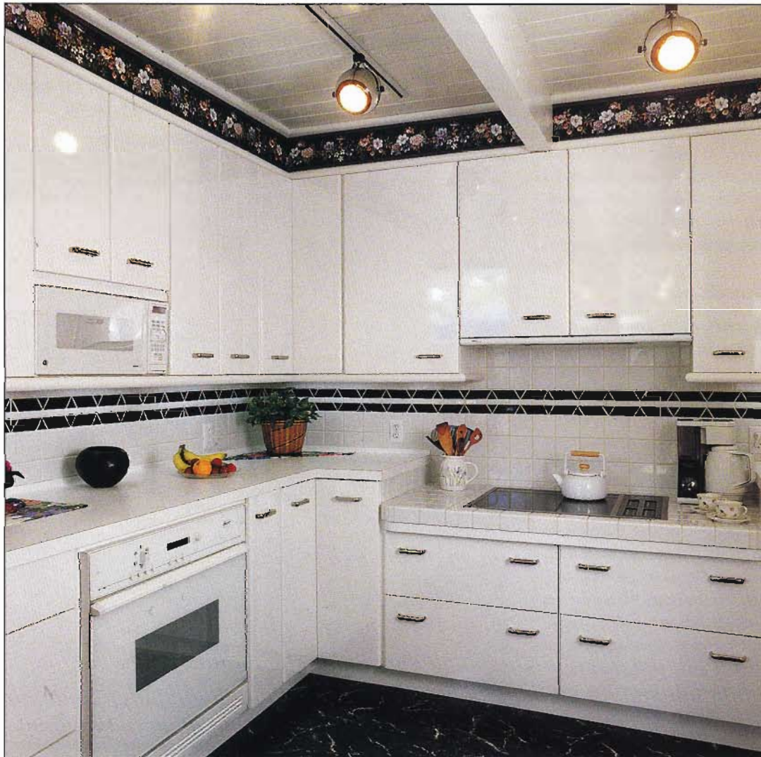
An induction cooktop, lowered here for convenience, offers the heating quality of gas without the fear of combustion. The glass burners magnetically heat metal only, while staying cool themselves, and the pots and pans then heat the food. A paper towel left on the functioning cooktop will not catch fire!
