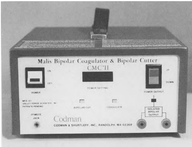
Fig. 18. The new solid state microprocessor controlled coagulator
