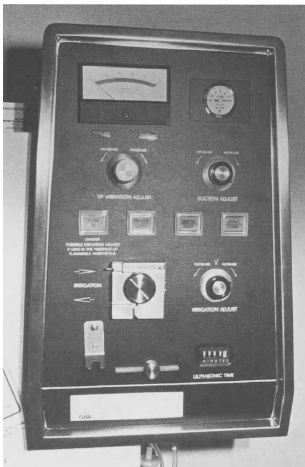
Fig. 7. Control panel of the Cavitron showing controls having vibration, suction and irrigation
