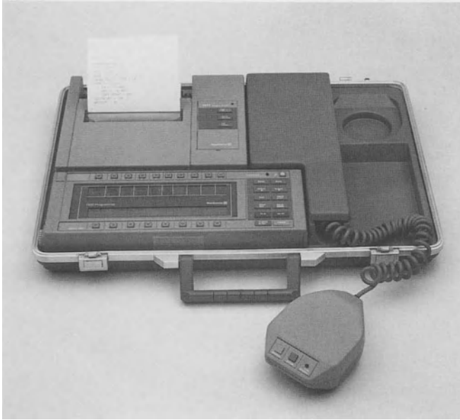
Fig. 9. Programmer for the ITREL totally implantable spinal cord or deep brain stimulation. Stimulation rate, amplitude, pulse width and length of on period of stimulation and off period between stimulation can be programmed transcutaneously and modified any time
