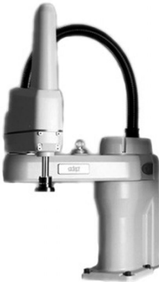
Figure 5.7. Example 5.3: Selective Compliant Articulated Robot for Assembly (SCARA). Adept model Cobra 600 (Courtesy of Adept Technology, Inc., Livermore, CA).
