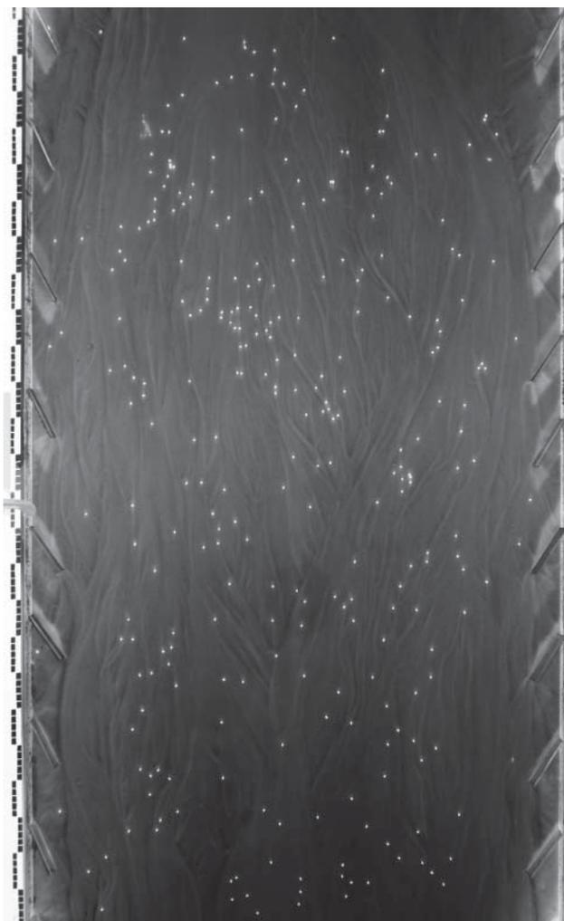
**Figure 20.7** Negative image of microscale experimental braidplain with plastic particles (in white) used to simulate logs dispersed randomly across the bed at the start of an experiment. Flow is from top to bottom. Scale along left edge denotes 1 cm and 5 cm increments.
