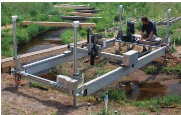
**Figure 20.5** Portable data acquisition (DAQ) cart ( $1.3 \times 3$  m) outfitted with an ultrasonic transducer to measure water surface, sonar to measure subaqueous topography and a downward-looking laser to measure above water topography. Individual cart locations are located using benchmarks and stitched together. Photograph courtesy Anne Lightbody, University of New Hampshire.
