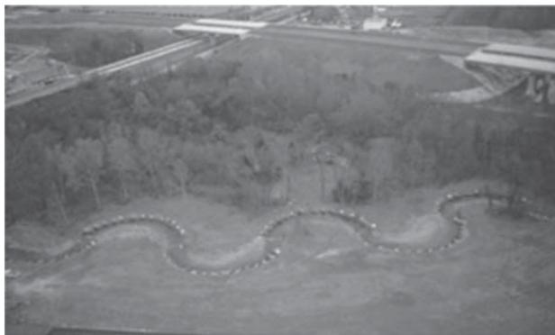
**Figure 7.14** Oblique aerial view of the Rosgen-type 'C-4' channel constructed on Deep Run, near Hanover, Maryland, shortly after construction in 1995. Source: Smith and Prestegard, 2005. Reproduced with permission of Wiley.
