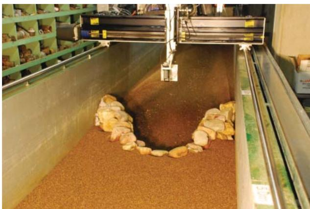
**Figure 20.2** An automated topography scanner from St Anthony Falls Laboratory capable of measuring  $150,000$  points  $s^{-1}$  to a resolution of  $0.3$  mm. The scanner is shown imaging the scour pattern around a rock structure similar to those installed in numerous restoration projects, from the channel shown in Fig. 20.1. Source: Craig Hill, Senior Research Associate, St Anthony Falls Laboratory.
