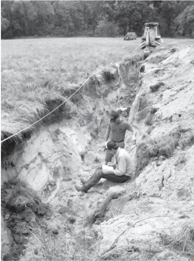
**Figure 2.5** Exploratory trench in floodplain alluvium, Big Piney Creek, Missouri. Source: US Geological Survey.
