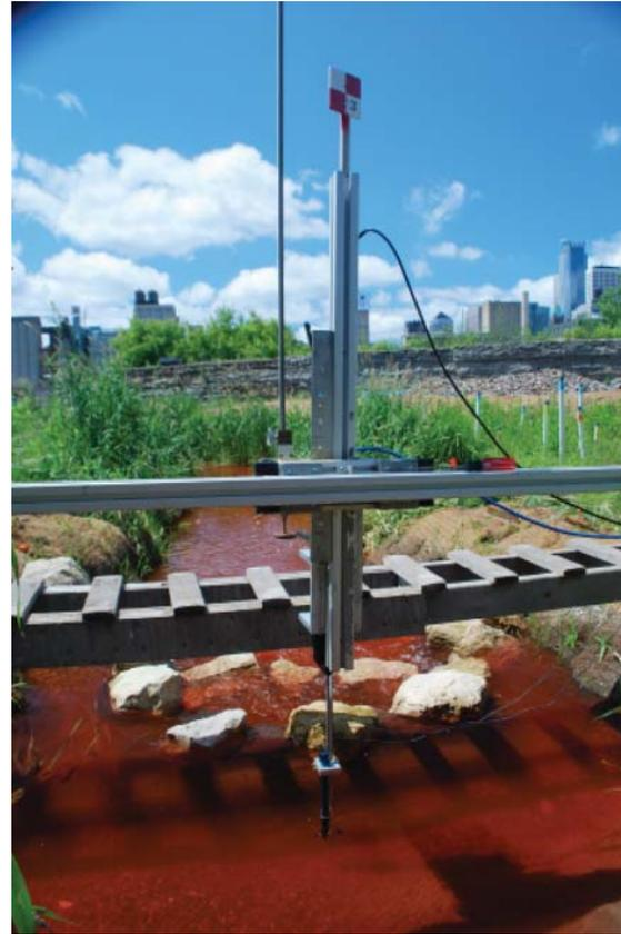
**Figure 20.11** Measuring simultaneous dissolved oxygen, temperature, nitrate and velocity in the vicinity of a rock structure in the SAFL Outdoor StreamLab.
