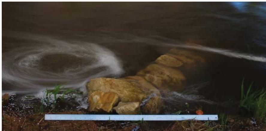
**Figure 20.9** Surface flow visualization in the OSL using white confetti and long-exposure photographs. Visualizations of this type provide a way of validating computational modelling results and provide insight into the complex flow patterns around instream structures. Flow is from right to left.
