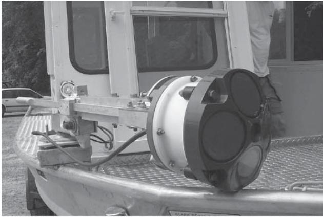
**Figure 12.5** Side and bottom view of an acoustic Doppler current profiler. Photograph courtesy of Robb Jacobson.
