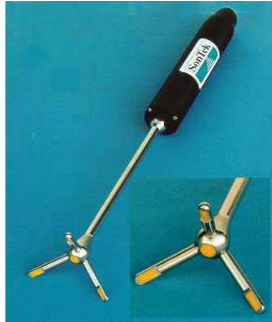
**Figure 12.4** Two views of an acoustic Doppler velocimeter. The larger view shows the probe and wand and the inset provides a close-up of the wand. Signals are emitted at the base of the wand and are received at the tips of each arm. The total spread of the arms is  $77\text{ mm}$ . Photograph courtesy of Sontek, Inc.
