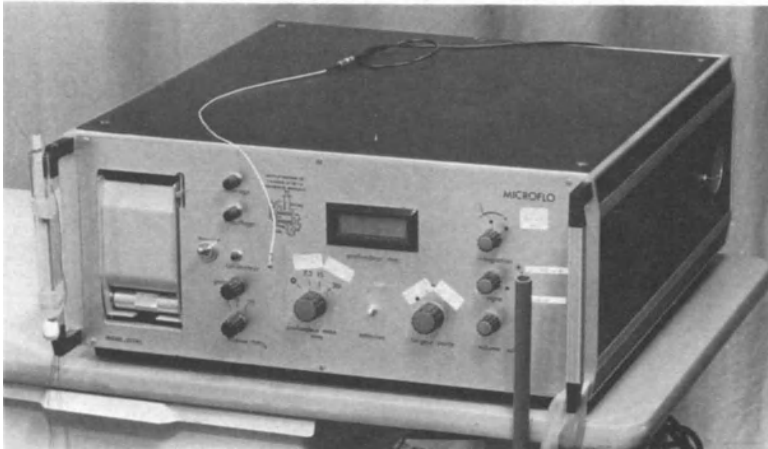
Fig. 1. 20 MHz pulsed ultrasonic velocity meter (Microflo) with probe
