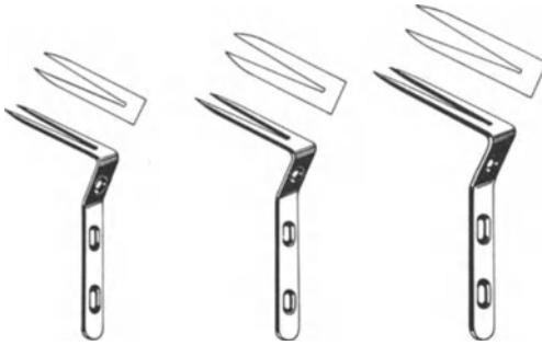
Fig. 3. The Altdorf hip clamp for intertrochanteric osteotomy in childhood. The clamp is available in 3 sizes. The proximal end of the blade is bifurcated and the blade itself is bent to make an angle of 130^\circ with the plate
