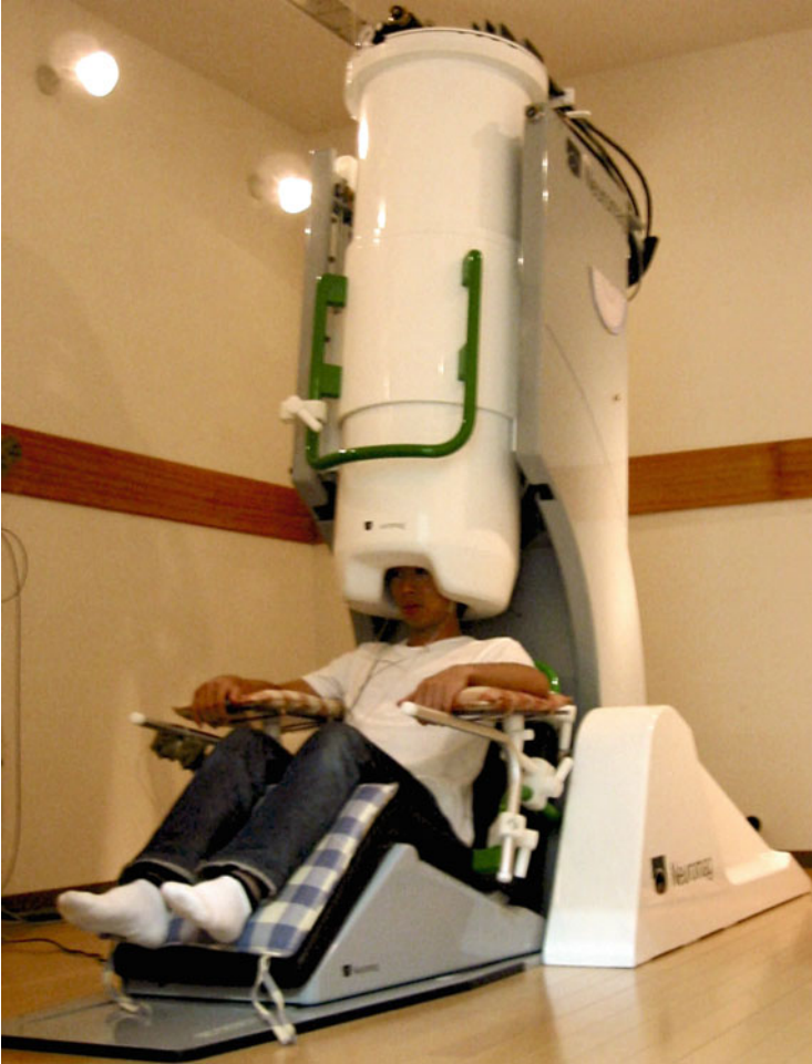
Photo 2.1 Magnetometer used in recording the magnetoencephalogram (MEG)
