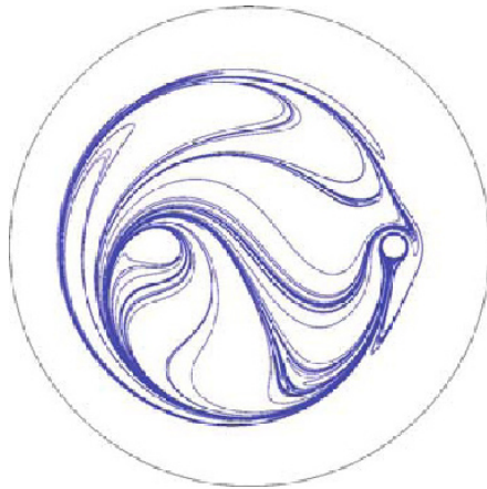
Figure 1. A material line being stirred by a moving rod in a viscous fluid. The rod is the circle visible in the centre-right portion of the fluid, but observe that there is a rod-like structure in the centre-left portion. This is a periodic island that acts like a rod—a ghost rod.
