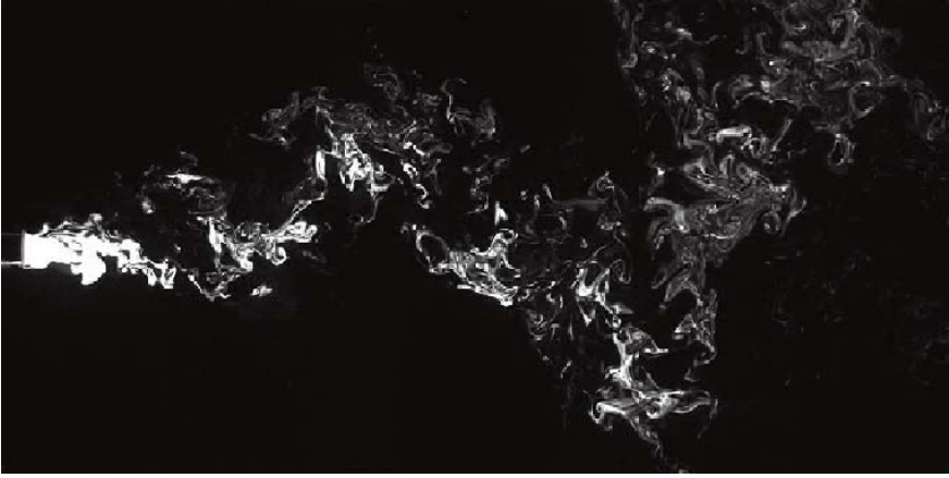
Figure 3. A snapshot of a dispersing plume made by the injection of a dye through a small tube of d = 8 mm in diameter on the axis of a larger turbulent jet whose integral scale is L = 8 cm at the injection location. Re = u'L/\nu = 10^4 .
