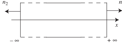
Figure 4.6 Schematic drawing of the closed surface to compute used the flux of \mathbf{J} : n_1 and n_2 are two versors. Transmitted and reflected currents contribute positively to the flux, whereas the incident current contributes negatively.
