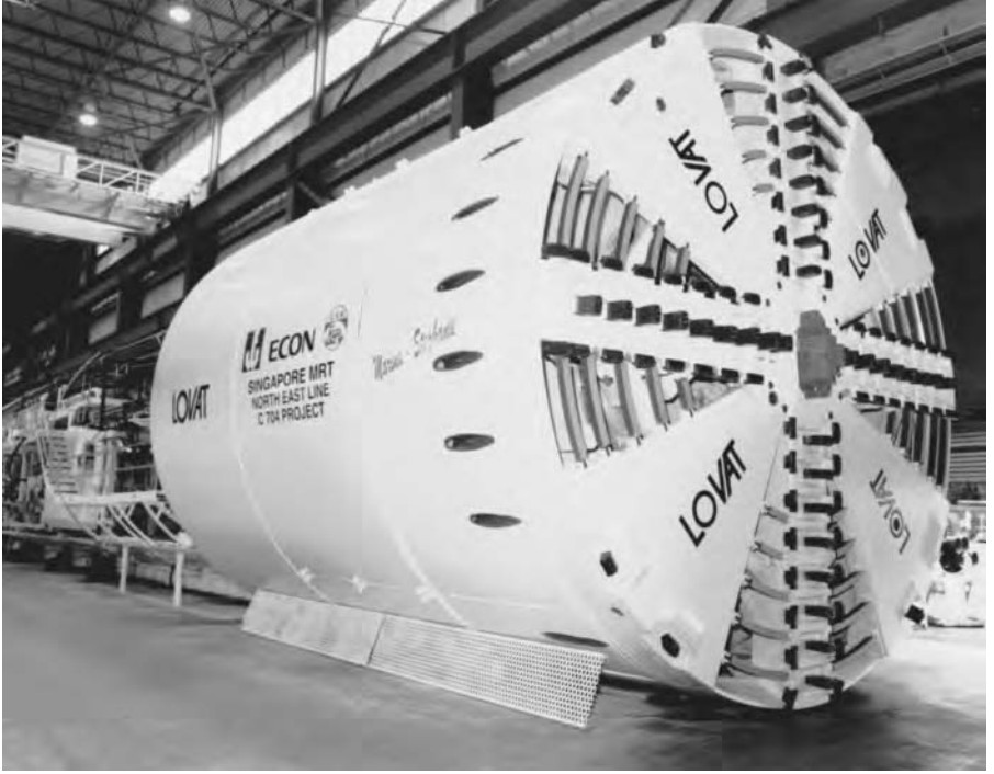
Figure 3.9 Earth Pressure Balance Shield cross-section.
