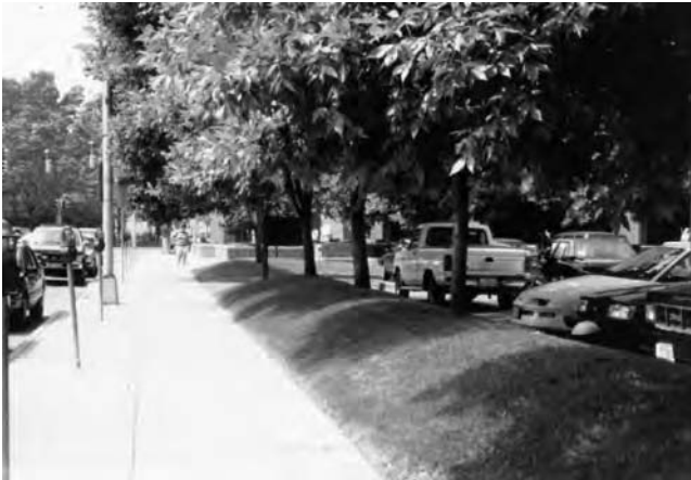
Figure 13.2 Berms can be used for screening or to gain soil volume in narrow spaces designated for planting. (Photo credit: N. Bassuk.)
