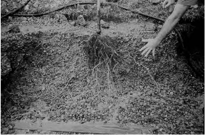
Figure 13.27 CU Soil test profile showing three years of root growth. Note the downward growth habit of the crabapple root system. This profile was paved as a sidewalk for field testing of the material in early research testing.
