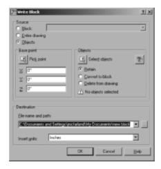
FIGURE 7.45: The Write Block dialog box
