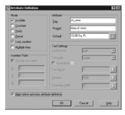
FIGURE 9.13: Setting the proper values in the Attribute Definition dialog box
