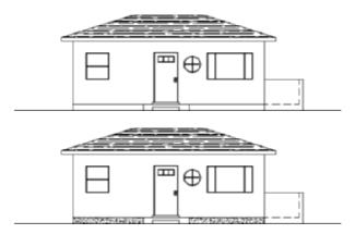
FIGURE 11.6: The front elevation with foundation lines drawn (top) and the resulting hatches in place (bottom)
