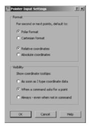
FIGURE 3.16: The Pointer Input Settings dialog box
