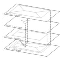
FIGURE 6.2: Separate layers combined to make a drawing
