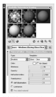
FIGURE 17.15: Adjusting the glass material in the Materials palette
