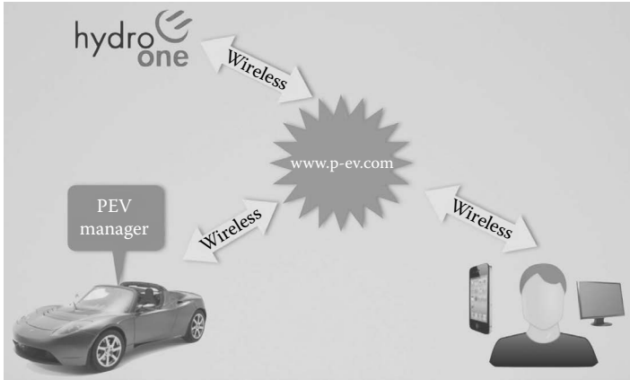
FIGURE 13.5 Wireless connectivity to the PEV as implemented at Ryerson Communications Laboratory.
