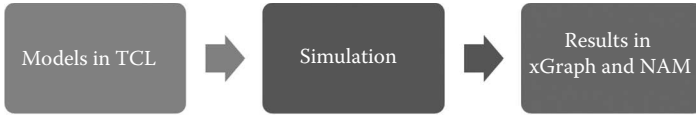
FIGURE 5.6 ns-2 flow. (Tcl, originally from tool command language is a scripting language. xGraph is a plotting program and Nam a Tcl/Tk-based animation tool.)
