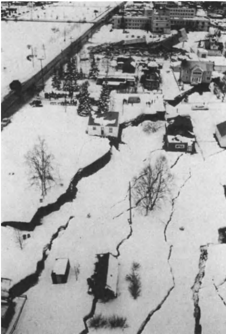
Figure 3.10. Anchorage, Alaska: Aerial View Showing Landslide Area after Earthquake of March 27, 1964. NOAA/EDIS.
