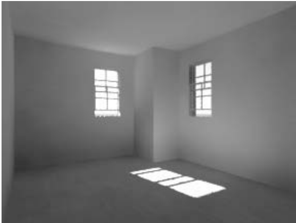
Turning on final gather in the mental ray render will generally give you excellent results for bounced light
