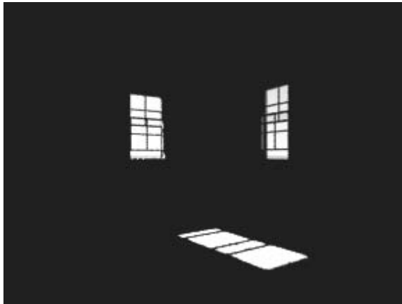
When Raytraced shadows are turned on and final gather is turned off, light entering into a room will produce a bright area in an overall dark space
