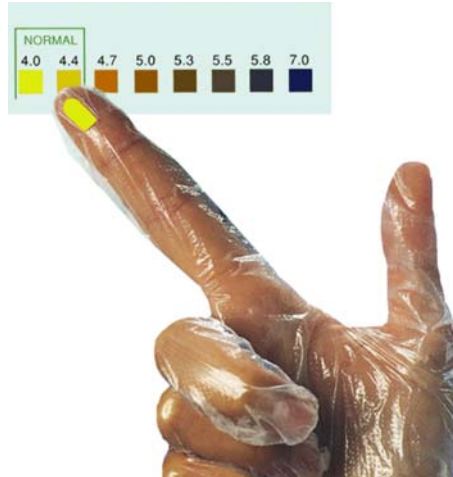
Figure 4. pH measurement: comparison with the color scale.
