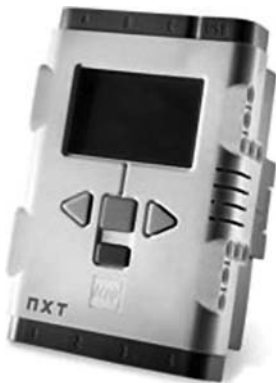
FIGURE 8.108 Lego Mindstorms™ NXT “brick.” (LEGO® and LEGO® Mindstorms® NXT™ are trademarks of the LEGO® Group, which does not sponsor nor endorse this book. This photo of the LEGO® Mindstorms® NXT™ brick is used here with permission. © 2010 The LEGO® Group.)
