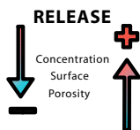
Fig. 7. Factors influencing the release of antibiotic from a PMMA matrix
