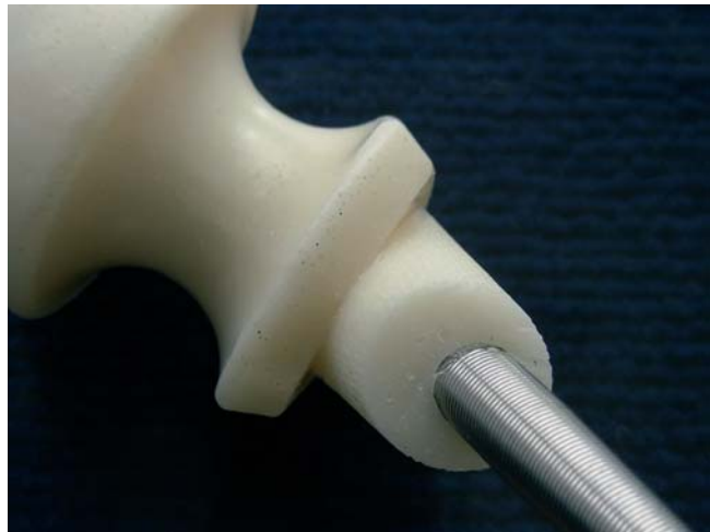
Fig. 2. Inner core present in Spacer-G
