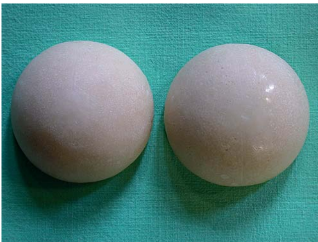
Fig. 5. Left: The head of the untested spacer. Right: The head of the spacer which completed the wear test. This head appeared smoother than the untested one due to polishing of the matching surface caused by abrasive wear.
