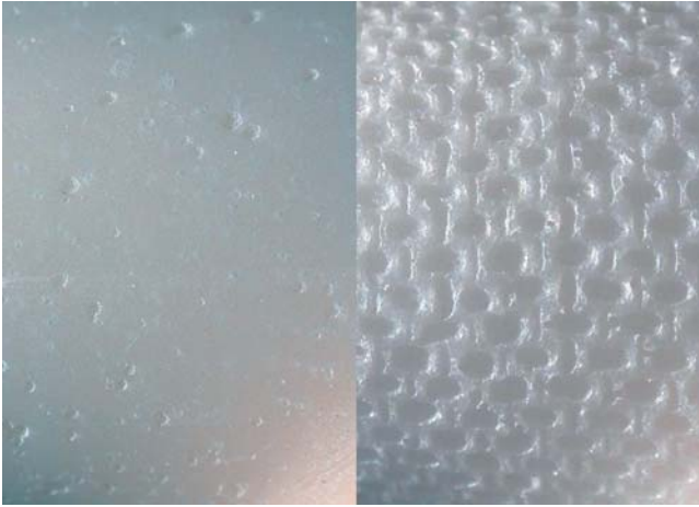
Fig. 9. Spacer-G stem: left, old version with smooth surface; right, new version with textured surface
