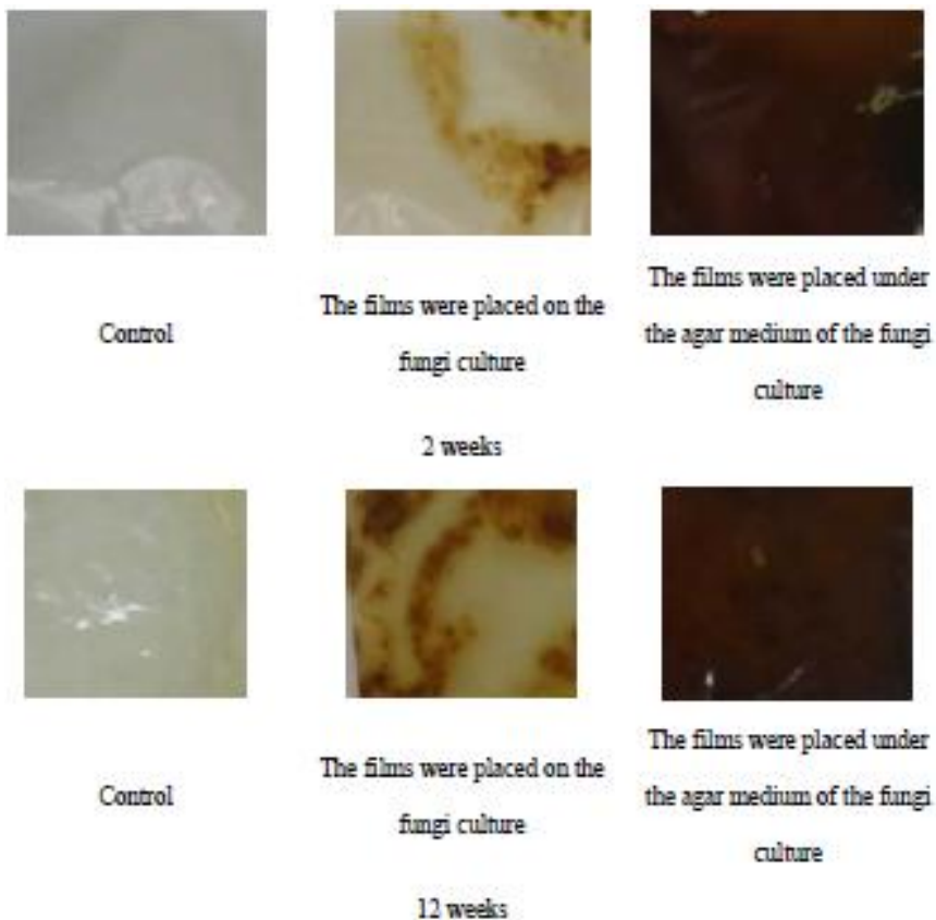
Figure 3. The photographs of the films in 2 and 12 weeks after A.terreus inoculation.
