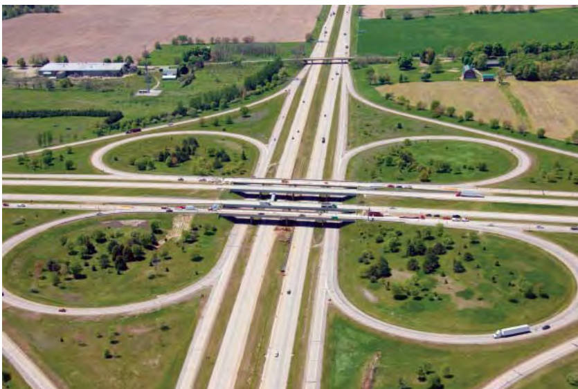
Figure 10-28. Four-Leg Interchange, Cloverleaf with Collector-Distributor Roads
