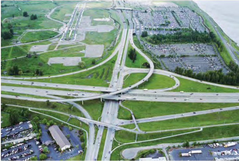
Figure 10-40. Four-Leg Interchange, Diamond with a Direct Connection
