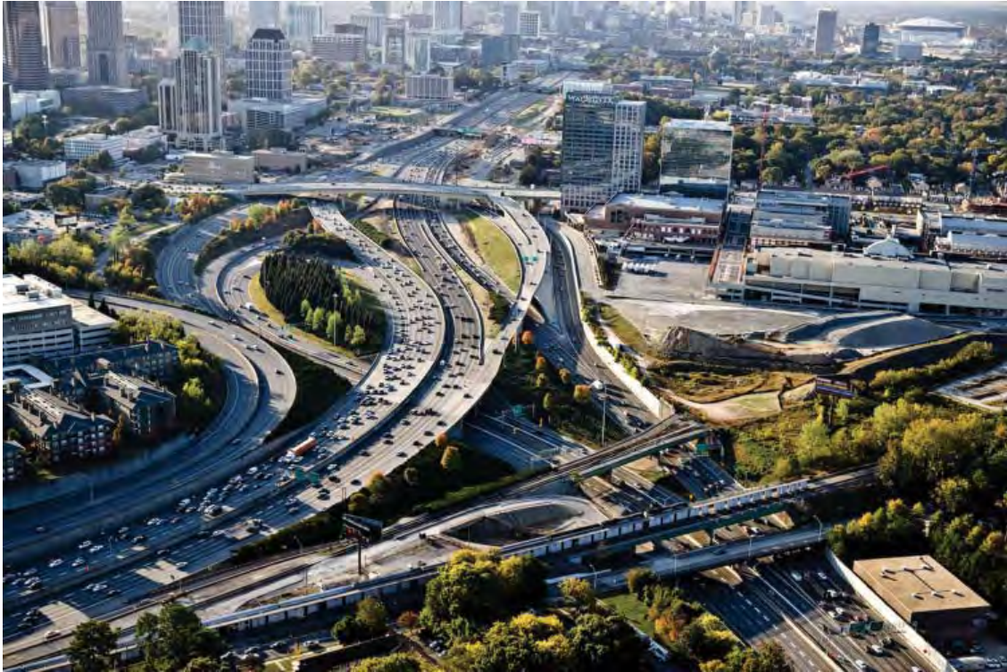
Figure 10-43. Complex Interchange Arrangement
