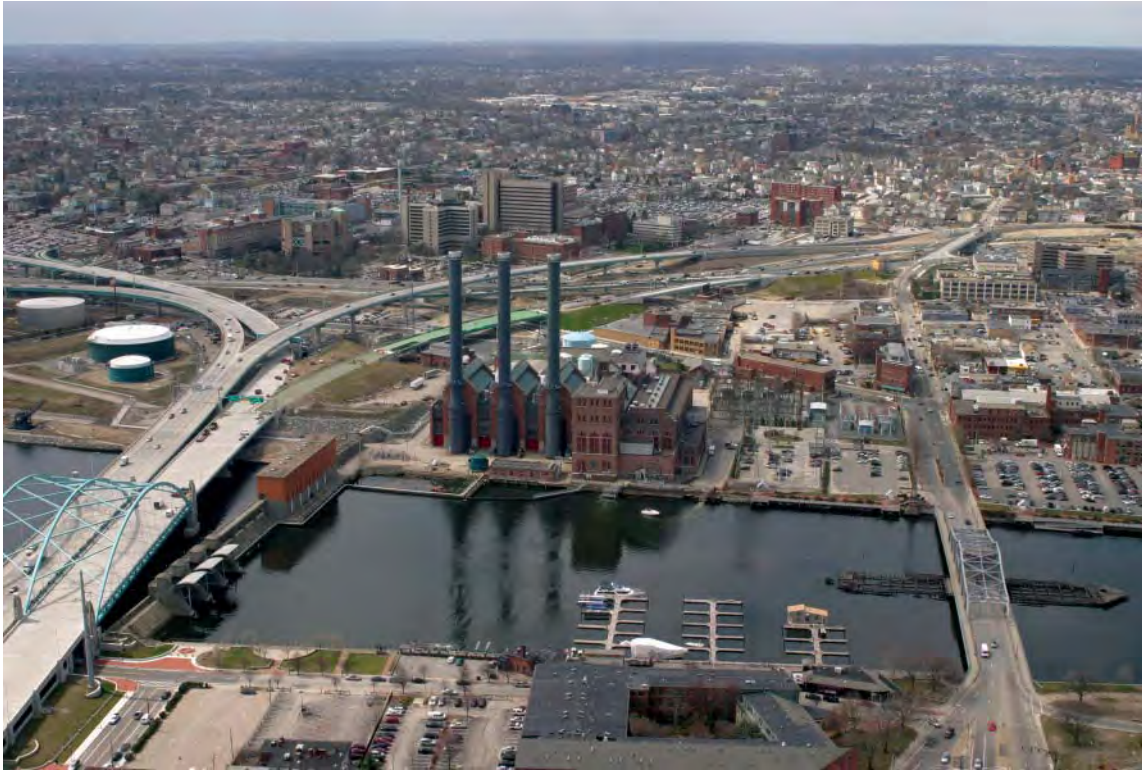
Figure 10-13. Directional Three-Leg Interchange at a River Crossing
