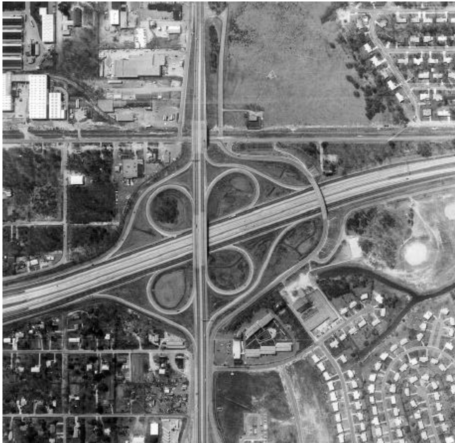
Exhibit 10-27. Cloverleaf Interchange With Collector-Distributor Roads
