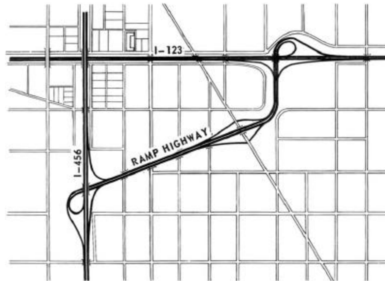
Exhibit 10-38. Offset Interchange via Ramp Highway
