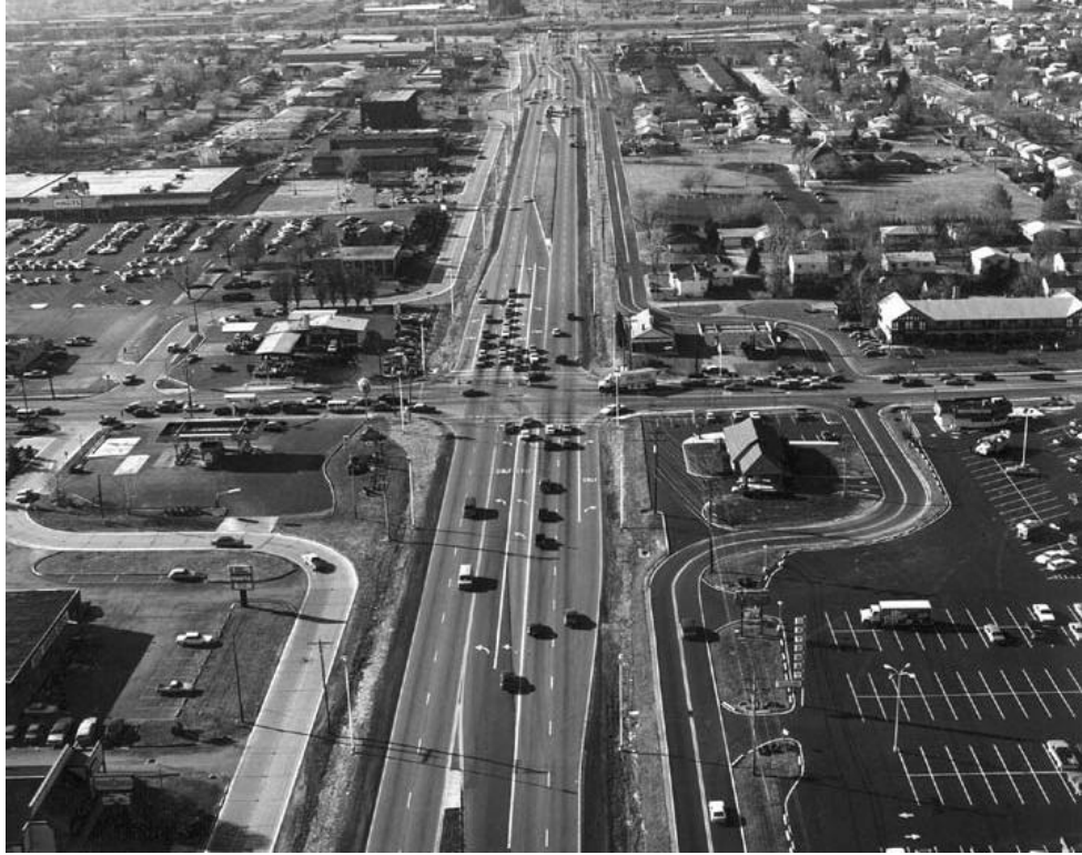
Exhibit 7-16. Divided Arterial Street With Two-Way Frontage Road
