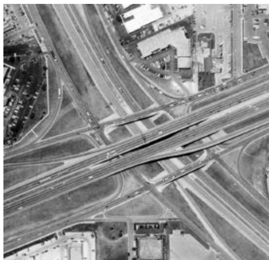
Exhibit 10-19. Freeway With a Three-Level Diamond Interchange
