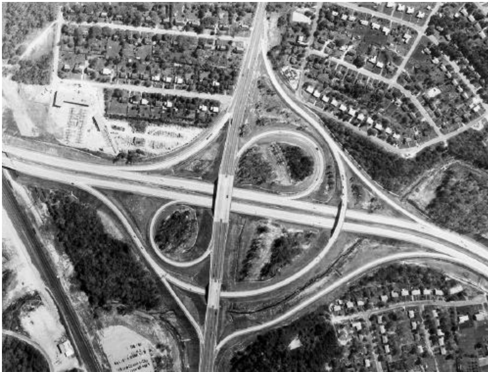
Exhibit 10-37. Semidirectional Interchange With Loops
