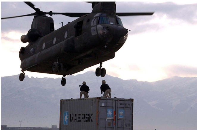
FIGURE 1.3 Chinook transport helicopter—payload 12,000 kg; range 1,100 km.
