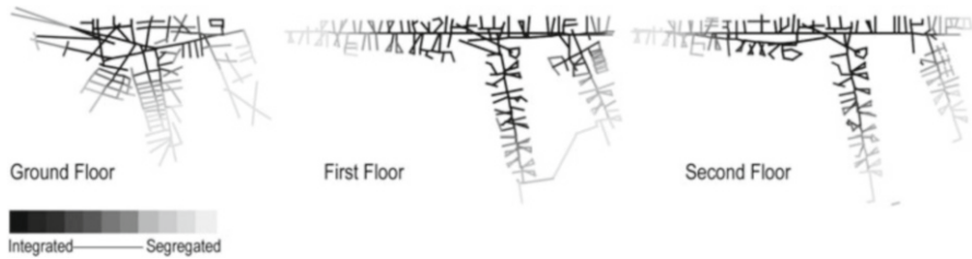
Fig. 7.6 Metric integration showing the spatial configuration of the research institute. Darker segments depict more integrated areas; brighter segments depict less integrated areas of the office
