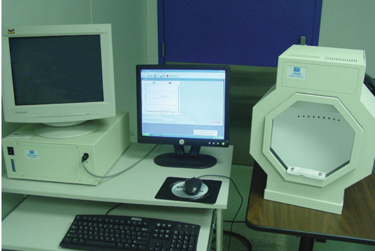
Fig. 4.2 Electroretinograph with full-field photostimulator noted on the right. The animal's head is placed in the photostimulator to achieve uniform flash illumination and maximal efficiency for retinal stimulation
