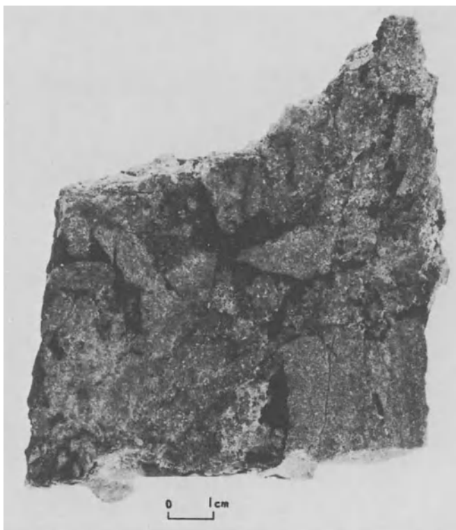
Fig. 7. Chalcocite ( black ) and chalcopyrite ( light grey ) ore in brecciated Pandurra Formation, Cattle Grid mine, Mount Gunson
