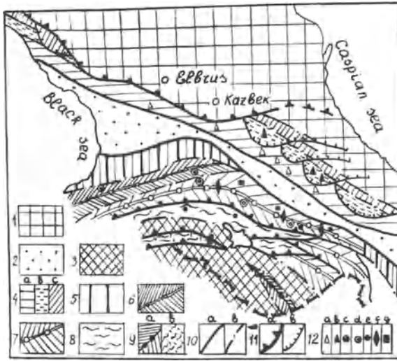
Fig. 1. Location of copper-lead-zinc deposits in the Alpine zones of the Caucasus. 1 Scythian craton; 2 Transcaucasian median mass; 3 Iranian median mass; 4 structural-formational zones of the Great Caucasus terrigenous eugeosyncline: a Psheki-Dagestan zone of early stabilization; b Bzyb-Tfan trough zone (central); c Chkhalt'a-Saryb'ash zone of the continental rise. 5 Adjar-Trialeti and Talysh superimposed troughs; 6 cretaceous volcanogenic island arc of Pontid; 7 Jurassic Somkheti-Kafan island arc; 8 Sevan-Akerin ophiolitic zone; 9 activated areas of the Iranian median mass: a Ordubad volcanogenic trough; b Vedi ophiolitic zone of the Cretaceous. 10 Boundaries of structural-formational megazones ( a ) and zones ( b ). 11 Alpine-type regional ( a ) and local ( b ) trusts. 12 Commercial-genetic types of deposits: a stratiform pyrite-base metal; b pyrite-chalcopyrite-pyrrhotite; c copper-pyrite; d pyrite-barite base metal; e sulfur-pyrite; f vein base metal; g copper-porphry
