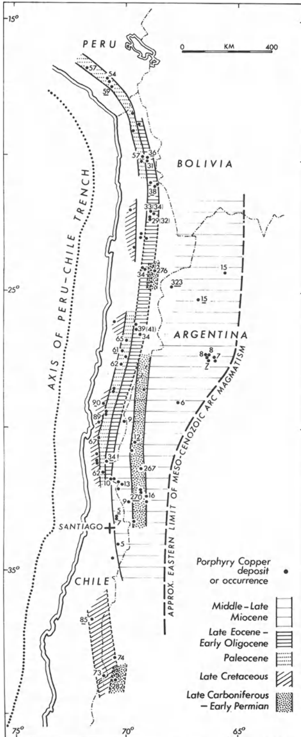
Fig. 3. Porphyry copper subbelts in the central Andes. All porphyry copper centres and breccia pipes from Fig. 2 are represented by dots. Numbers refer to K-Ar ages determined on hydrothermal or, where underlined , magmatic minerals. Numbers in parenthesis are alternative ages. K-Ar dates given to nearest m.y.; where more than one apparently reliable date is available, an average is given. Data sources are detailed in Sillitoe (1981), except for new determinations for Quebrada Blanca (Hunt et al. 1983), La Escondida (Minera Utah de Chile, Inc., unpublished data 1983), Domeyko (Shell Chile, unpublished data 1983), El Indio (Araneda 1982), Disputada (Warnaars 1983), and Estero San José and Galletué (Alfaro 1980)
