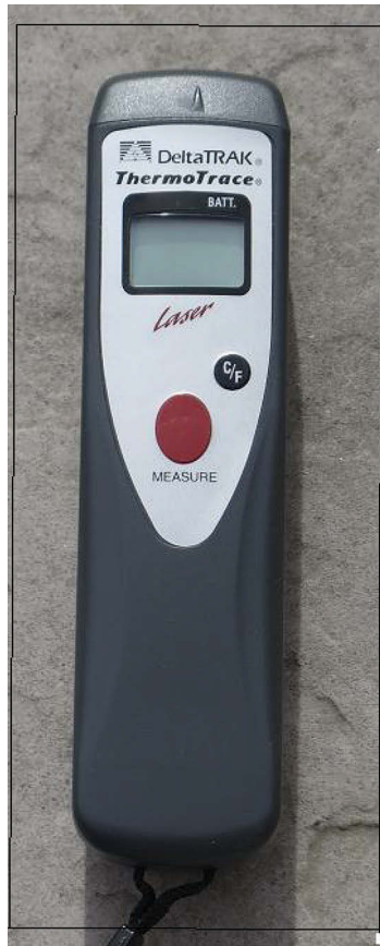
Figure 8.4 Noncontact digital thermometer. (From Author's Collection.)
