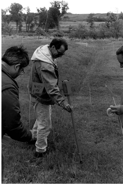
Figure 7.6 Valve and box locator. (From Author's Collection.)
