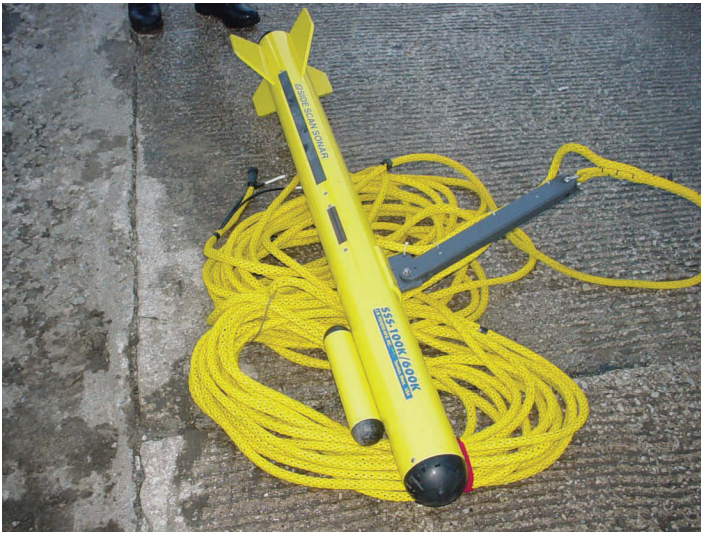
Figure 9.1 Side-scan sonar. (From Author's Collection.)
