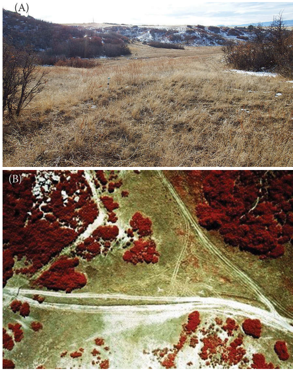
Figure 8.3 Natural color image: (A) false-color infrared image and (B) Necro-Search research site. Note: In (B) the red color indicates healthy vegetation, while the brown area, left center, indicates disturbed vegetation (grave sites of three pigs.) (From Author's Collection.)
