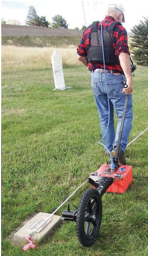
Figure 6.3 Radar profiling systems, GSSI pulled system with distance wheel. (Courtesy of Rockware.)
