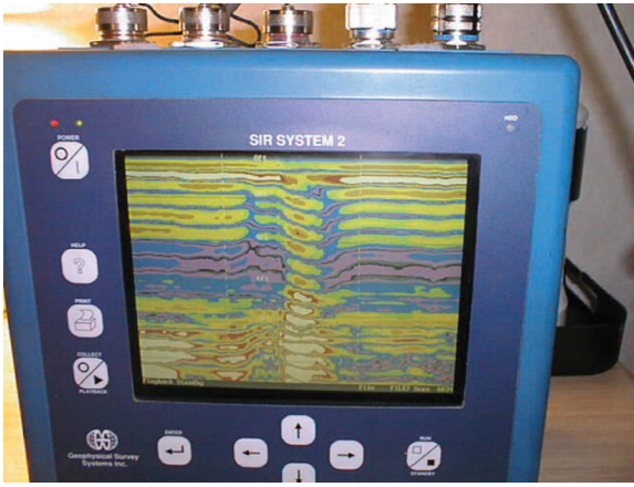
Figure 6.4 GPR profile, on GSSI monitor.
