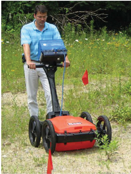
Figure 6.2 Radar profiling systems, GSSI cart-mounted system. (Courtesy of Geophysical Survey Systems, Inc.)
