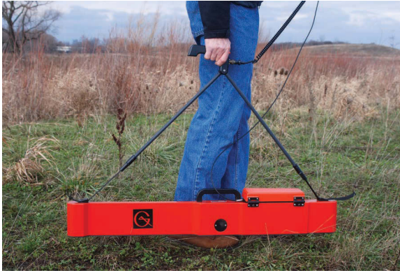
Figure 5.2 Ground conductivity meter, Geonics EM38 with extender arm. (Courtesy of Geonics Limited.)
