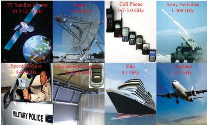
Figure 6.1 Examples of radio-frequency interference sources from human activities including communication satellite, radar, cell phone, vehicle speed monitor, and garage door opener.
