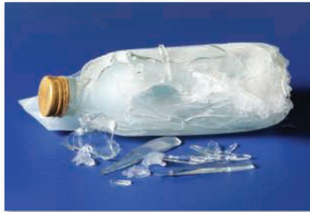
Figure 2.15 Ice breaks bottle The bottle broke because water expands about 9 percent when it freezes. (Photo by Martyn F. Chillmaid/Science Source)
