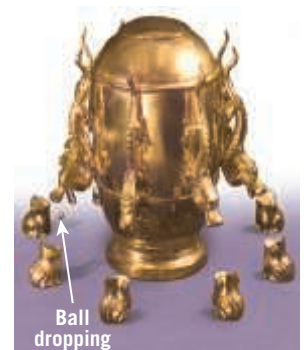
Figure 6.7 Ancient Chinese seismograph. During an Earth tremor, the dragons located in the direction of the main vibrations would drop a ball into the mouth of a frog below. (Photo by James E. Patterson Collection)
