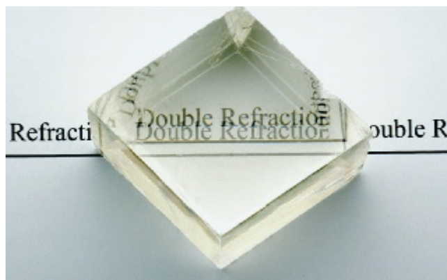
Figure 1.19 Double refraction This sample of calcite exhibits double refraction. (Photo by Chip Clark/Fundamental Photographs)
