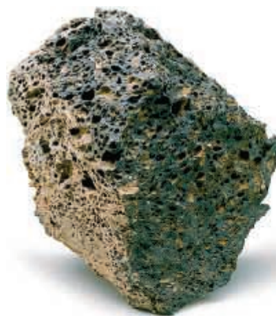
A. Scoria is a vesicular rock commonly having a basaltic composition. Pea-to-basketball size scoria fragments make up a large portion of most cinder cones (also called scoria cones).
