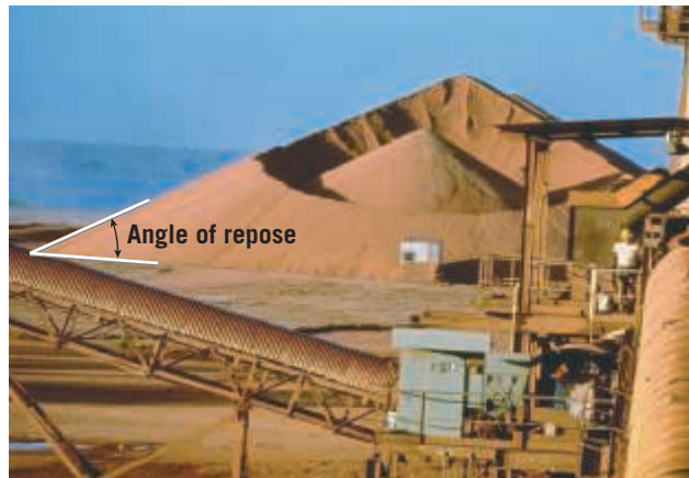
Figure 3.5 Angle of repose The angle of repose is the steepest angle at which an accumulation of granular particles remains stable. Larger, more angular particles maintain the steepest slopes. (Photo by George Leavens/Science Source)
