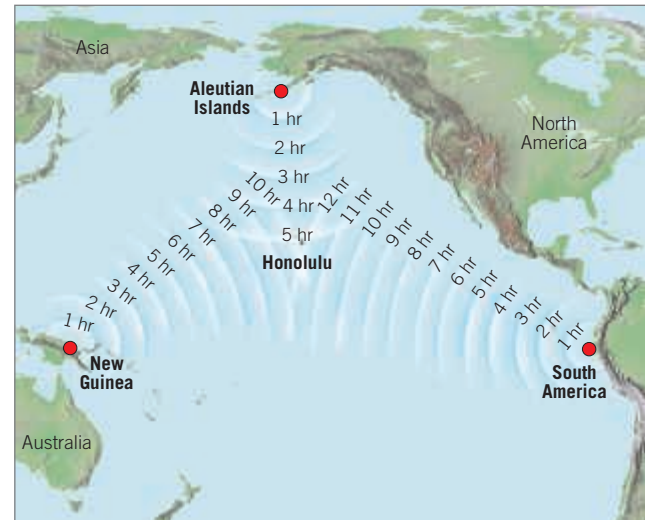
Figure 6.32 Tsunami travel times Travel times to Honolulu, Hawaii, from selected locations throughout the Pacific. (Data from NOAA)
