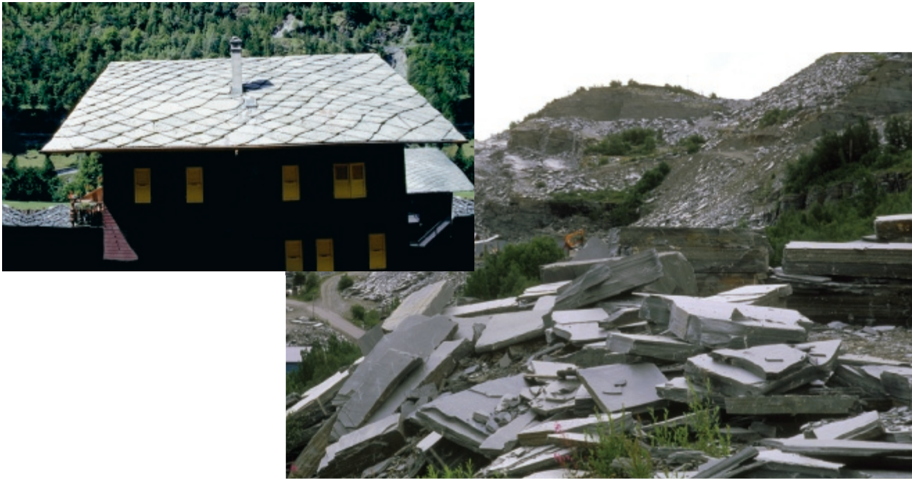
Figure 2.34 Slate exhibits rock cleavage. Because slate breaks into flat slabs, it has many uses. The larger image shows a quarry near Alta, Norway. (Photo by Fred Bruemmer/Getty Images) In the inset photo, slate is used to roof a house in Switzerland. (Photo by E. J. Tarbuck)
