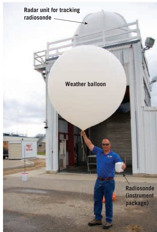
Figure 11.10 Radiosonde A radiosonde is a lightweight package of instruments that is carried aloft by a small weather balloon. It transmits data on vertical changes in temperature, pressure, and humidity in the troposphere. The troposphere is where practically all weather phenomena occur, so it is very important to have frequent measurements. (Photo by David R. Frazier/Danita Delimont/Newscom)
