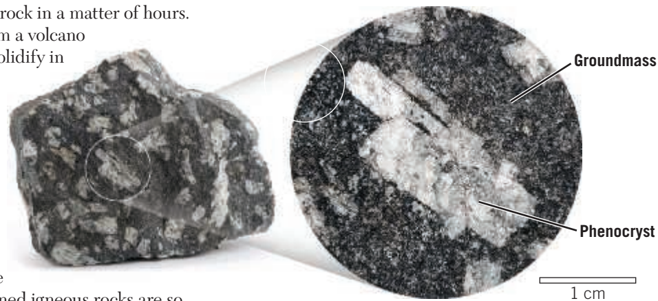
Figure 2.5 Porphyritic texture The large crystals in porphyritic rocks are called phenocrysts , and the small crystals constitute the groundmass . (Photos by Dennis Tasa)
