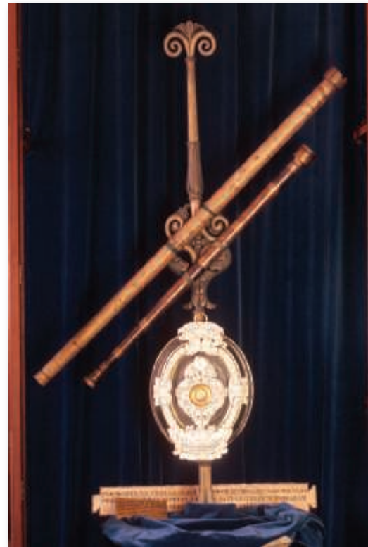
Figure 15.12 One of Galileo's telescopes Although Galileo did not invent the telescope, he built several—the largest of which had a magnification of 30. (Photo by Gianni Tortoli/Science Source)
