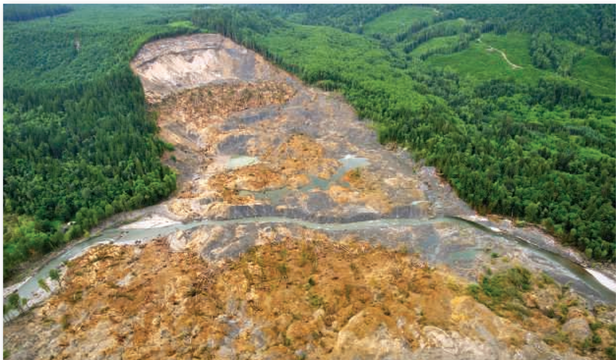
Figure I.11 Deadly debris flow This image provides an example of interactions among different parts of the Earth system. Extraordinary rains triggered this debris flow (popularly called a mudslide) on March 22, 2014, near Oso, Washington. The mass of mud and debris blocked the North Fork of the Stillaguamish River and engulfed an area of about 2.6 square kilometers (1 square mile). Forty-three people perished. (Photo by Michael Collier)
