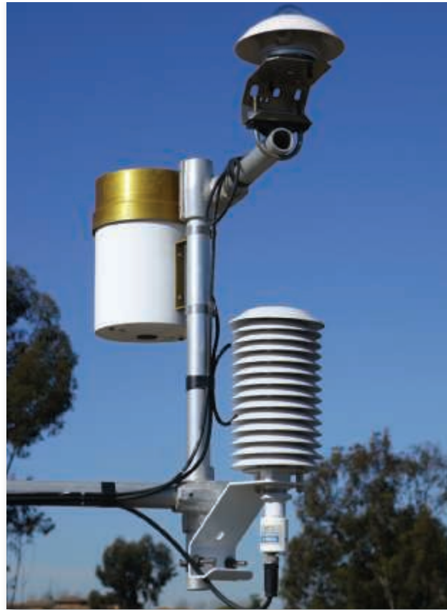
Figure 11.29 Measuring temperature electrically This modern shelter contains an electrical thermometer called a thermistor . A shelter protects instruments from direct sunlight and allows for the free flow of air. (Photo by GIPhotoStock/Science Source)
