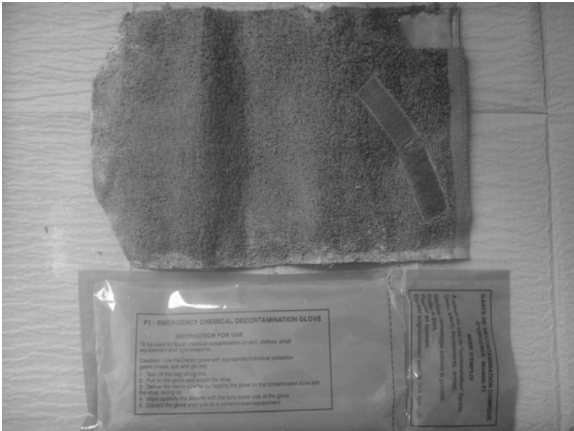
Fig. 18.3. French Army emergency decontamination kit: (a) sponge (glove external side); (b) Fuller's earth-containing porous fabric (glove internal side) (pictures by Dr Denis Josse).
