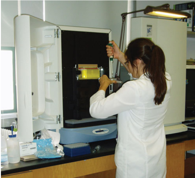
FIGURE 1.8 Student loading DNA samples into vertical gel on a LI-COR Biosciences 4300 DNA Analyzer. Photograph by Erin Sanders and Rachel Sauvageot (UCLA).
