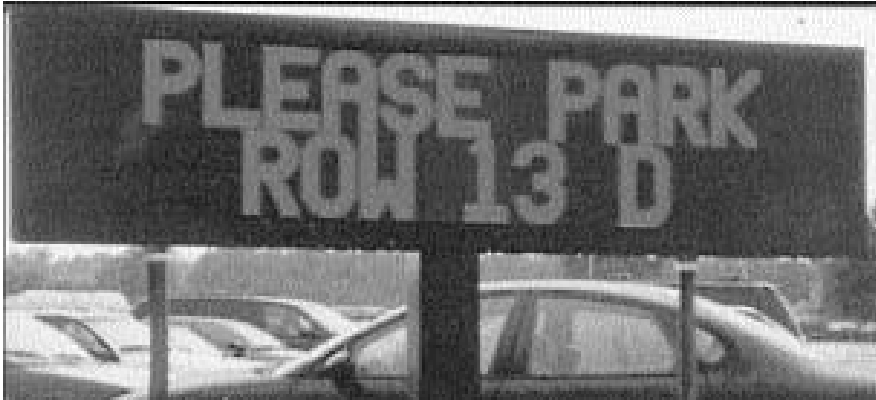
Figure 6-30. Smart parking facilities provide specific parking space availability.
