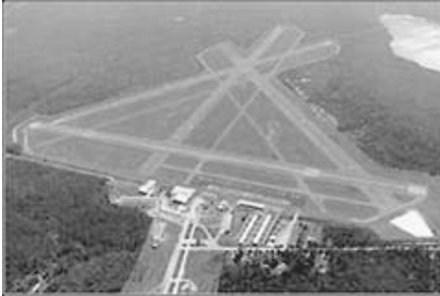
Figure 4-2. Flagler County Airport in Bunnell, Florida, has multiple crosswind runways to accommodate smaller aircraft in variable wind conditions. (Photo courtesy Seth Young)
