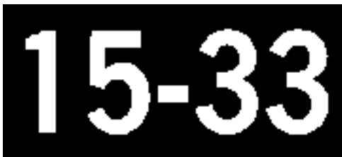
Figure 4-25. Runway holding position sign.
