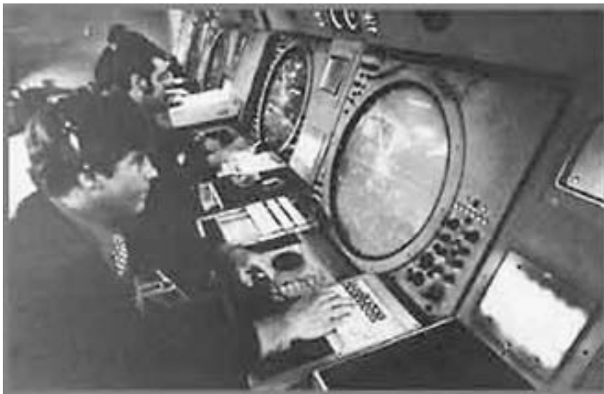
Figure 5-3. Automated Radar Traffic (ARTS) System at Jacksonville Center circa 1970. (Source: FAA)
