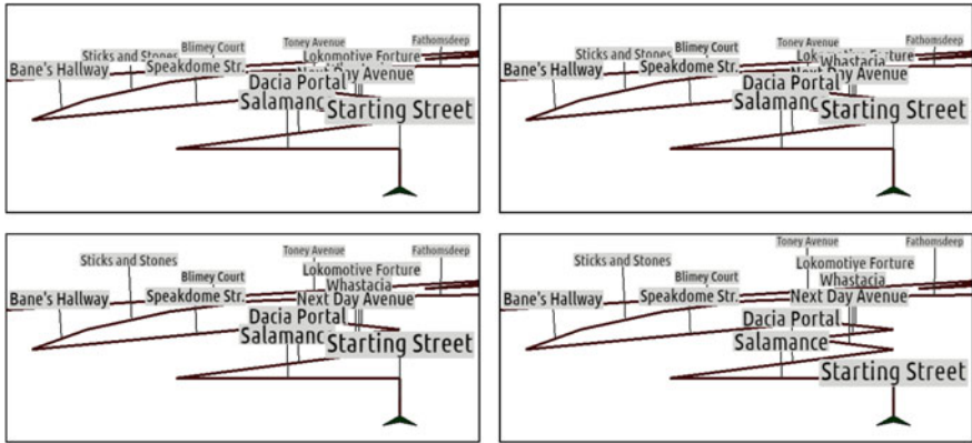
Fig. 8 Screenshots of our program in an artificial data set. In reading direction: Within 1.5 s, the overlap of the initial label placement is resolved. On the very first subfigure, the total overlap is 6773 pixels
