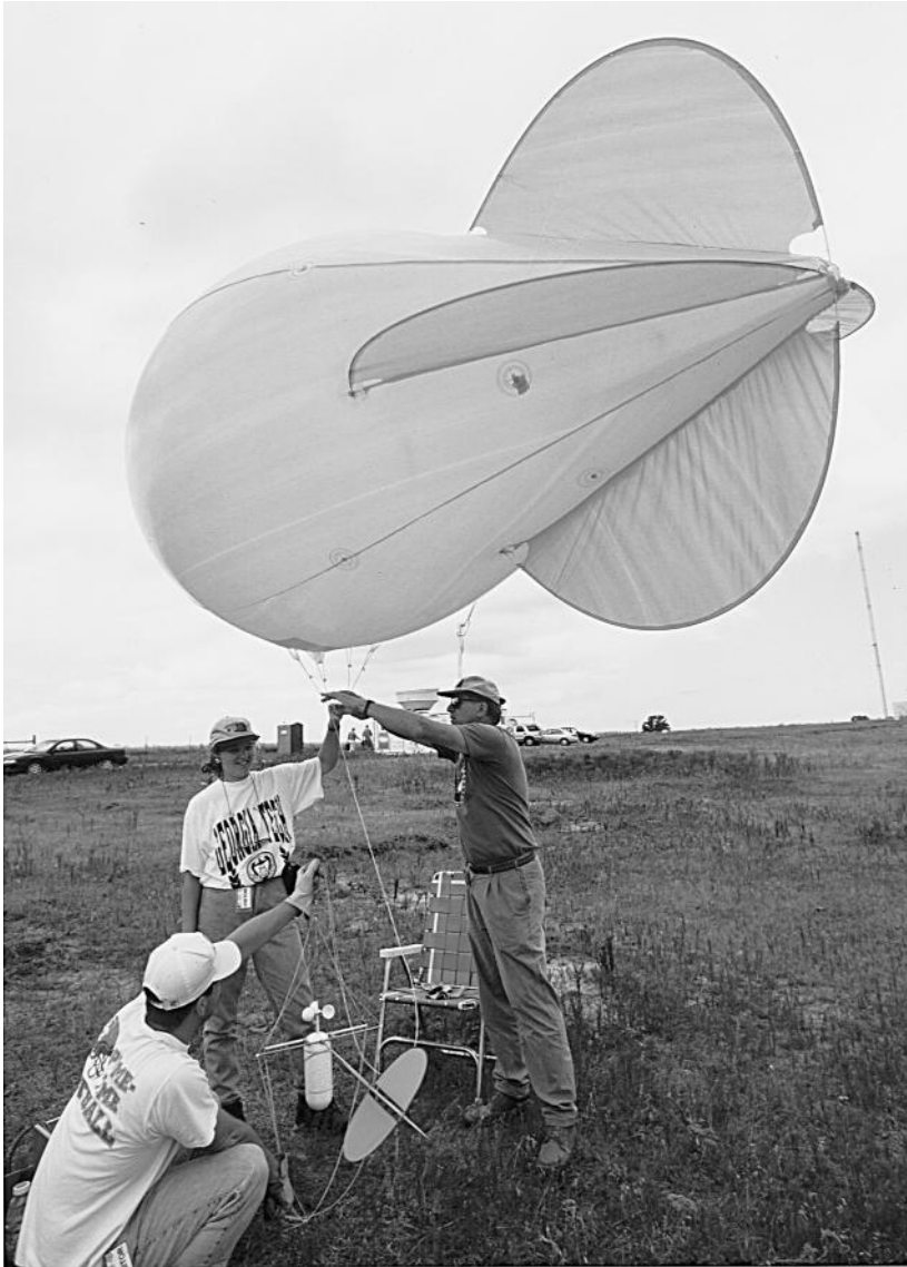
A physical meteorologist ( right ) from the National Severe Storm Laboratory, a professor, and a graduate student prepare to launch a tethered weather balloon carrying instruments that measure humidity, temperature, and wind speed. ( Jack Dykinga, Agricultural Research Service, USDA )
