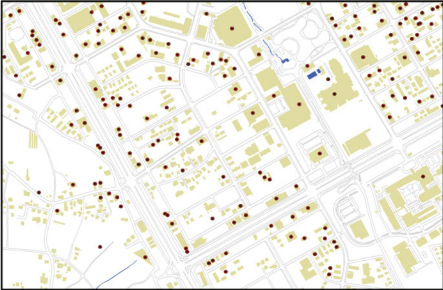
Fig. 6.5 NTT iTownpage point layer overlays on building footprints polygon layer to separate residential vs. non-residential buildings
