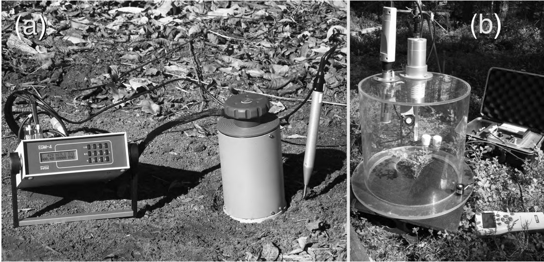
Figure 2.4 Closed chamber systems from different manufacturers (a) PP-Systems SRC-1 closed dynamic chamber, (b) Vaisala GMP-343 CO 2 probe connected to a closed chamber made by Tunkua Oy, Finland. In the figure, a transparent chamber is being used for measuring photosynthesis of ground vegetation.
