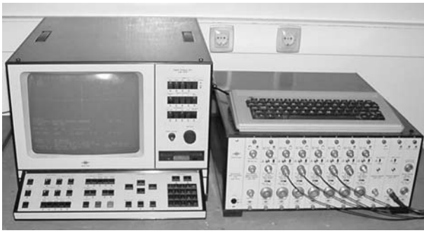
Figure 7 Example of multichannel FFT analyzer.
