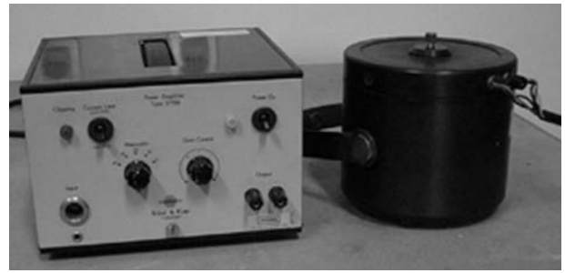
Figure 2 Example of electromagnetic exciter and matching power amplifier.
