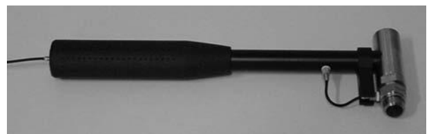
Figure 4 Impact hammer with force transducer and soft head.
