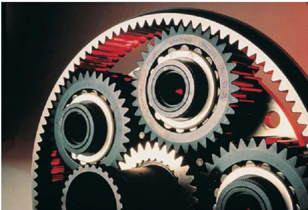
Plate 37 Gear Diagnostics. Gear from an aircraft. Part of the transmission system in an aircraft engine. This gear consists of flywheels with teeth which transmit rotating movements between shafts. (With permission from Science Photo Library).
