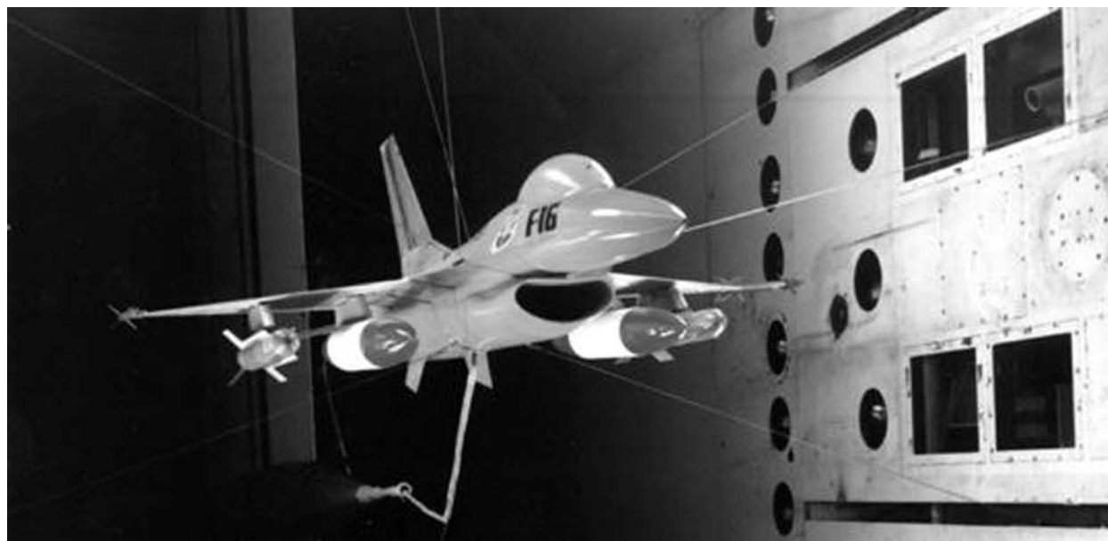
Figure 7 F-16 wind-tunnel model on the NASA Langley transonic dynamics tunnel two-cable mount system (courtesy of NASA Langley Research Center).
