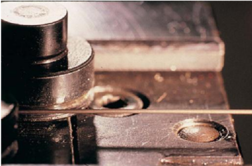
Plate 51 Shape Memory Alloys. Memory metal. Close-up view of a wire of memory metal being 'educated' by being bent around a spindle. Memory metals are alloys of nickel, titanium and aluminium or copper. Once manufactured in a certain shape the metal may be deformed with little effort, but will regain its shape upon gentle heating. The heat makes the metal plastic, allowing it to return to the structural arrangement in which it was made (its minimum energy configuration). Repeated bending of the metal, each time to the same position, alters the original structure permanently and 'educates' it to a new shape. (With permission from Science Photo Library).
