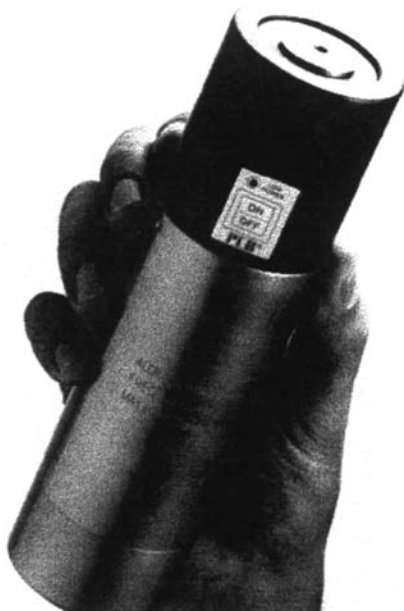
Figure 12 (A) Cross-section of accelerometers used in back-to-back calibration arrangement. (B) Photograph of a hand-held calibrator. Courtesy of PCB Piezotronics, Depew, NY.
