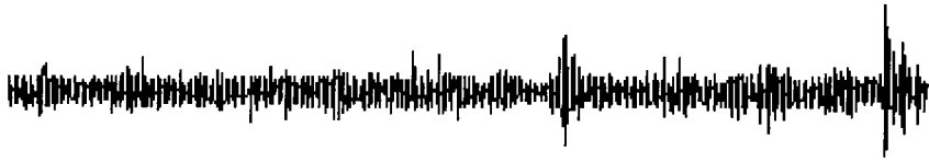
Figure 4 Bearing vibration with inner-race defect.
