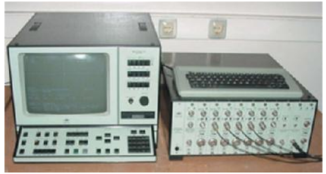
Plate 45 Modal Analysis, Experimental: Measurement Techniques. Example of multichannel FFT analyzer.
