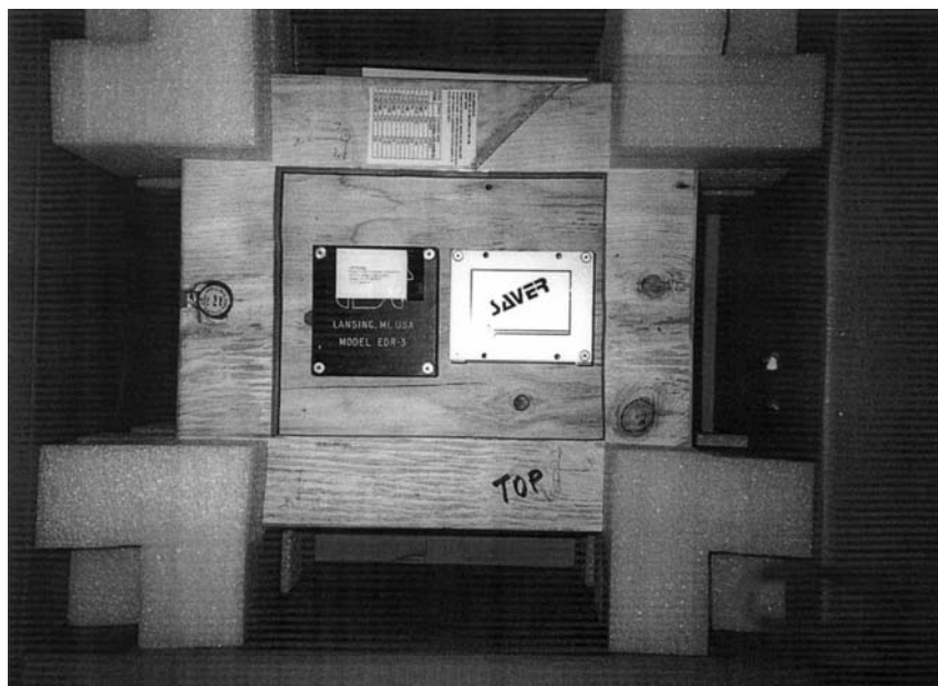
Figure 3 Monitoring the distribution environment with self-contained data acquisition instrumentation: (A) recording unit; (B) typical package configuration; (C) dummy package with the recording unit installed.
