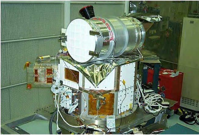
Figure 4. Scripps-EPIC on the DSCOVR Spacecraft.
