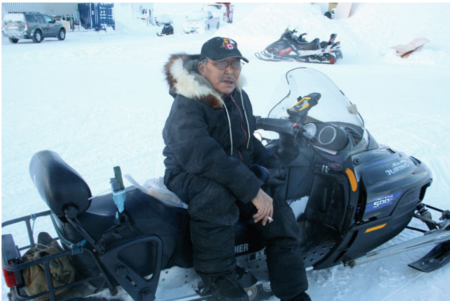
Fig. 8.5 Jacopie Panipak with the Igliniit system installed on his snowmobile. The PDA is mounted with ruggedized mounting hardware on his handlebars. The weather station is mounted at the back of the snowmobile. A serial cable connects the two units and weather data are stored automatically on the PDA (Photo: Shari Gearheard)
