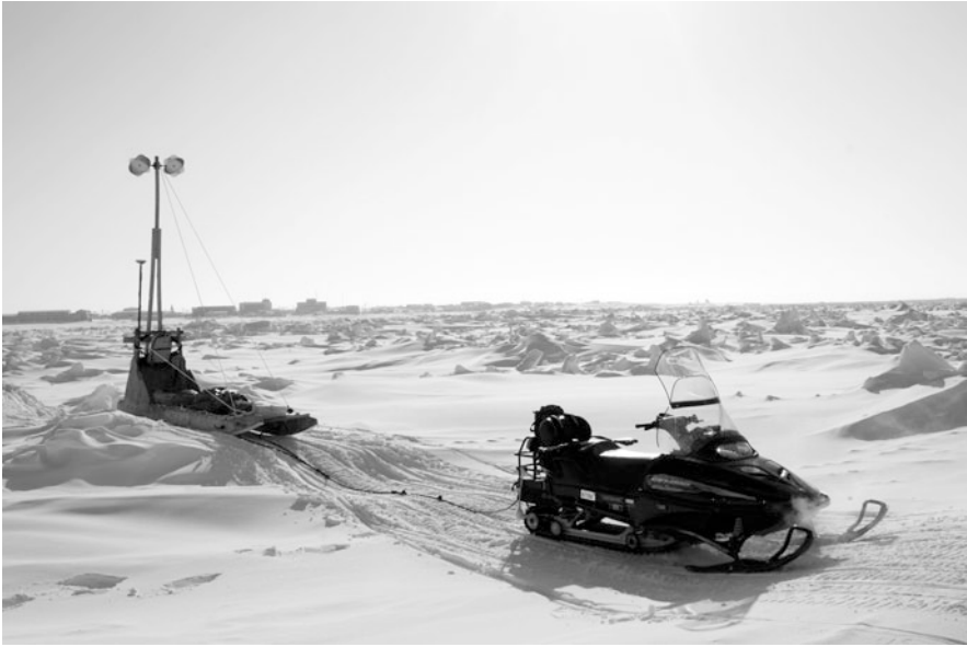
Fig. 9.8 Snowmobile hauling a sled with the ice survey instruments. Shown here is the EM31 conductivity meter that measures ice thickness, a highly accurate differential GPS, and a radar-reflector mast, which allows the measurements to be located in the imagery collected by the coastal radar in downtown Barrow (see Fig. 9.9). The skyline of Barrow can be seen in the distant background. (Photo: M.L. Druckenmiller)
