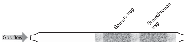
Figure 6.4 Two-section trap for Method 30B.
