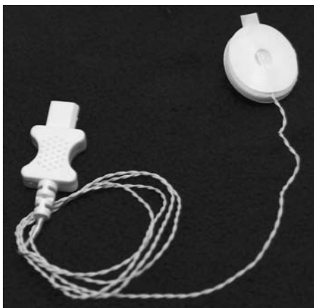
Figure 12 Skin surface temperature sensor with 400 series thermistor.
