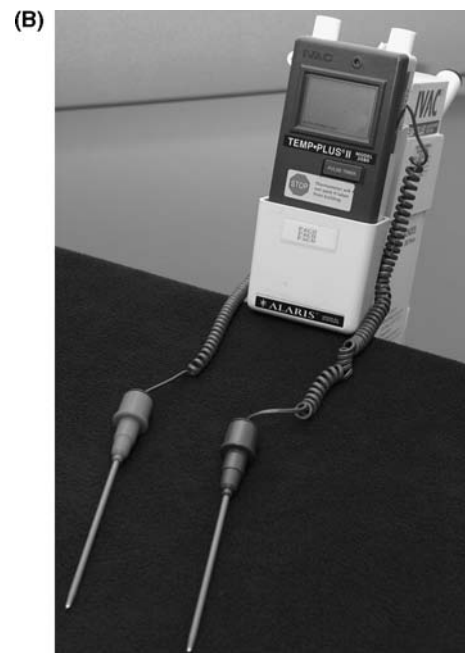
Figure 10 (A) and (B). An electronic thermometer can be used to accurately measure sublingual ( black probe ) or rectal ( gray probe ) temperatures (IVAC Temp Plus II, Model 2080, Alaris Medical, San Diego, California, U.S.A.).
