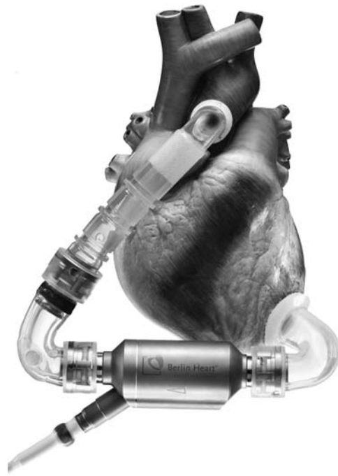
Figure 21 The Berlin Heart INCOR ® . Like the majority of the new axial flow VADs, the INCOR draws blood from the left ventricle apex and returns it to the ascending aorta. However, unlike all the other devices, the impeller is magnetically levitated. Without bearings, the durability of the device is likely to be very long, and the potential for thrombosis is markedly diminished. Source: Courtesy of Berlin Heart.
