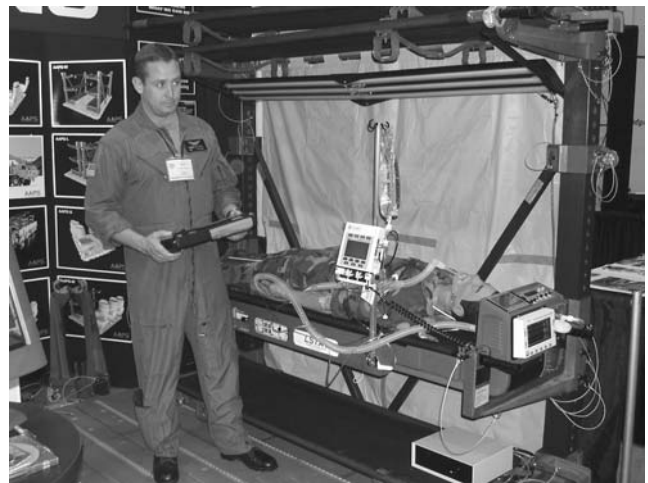
Figure 1 Life Support for Trauma and Transport (LSTAT ® ). The patented LSTAT system is an individualized, portable, networked ICU and surgical table in a patient-care platform. Integrated within the LSTAT system are a state-of-the-art defibrillator, ventilator, suction, three-channel fluid and drug infusion pump, point-of-care blood chemistry analyzer, and patient monitoring subsystems. The platform, which is only 5 inches thick, also incorporates on-board power and oxygen subsystems. The medical subsystems are further integrated into an on-board computer that captures, stores, and transmits continuous, real-time, multi-device, multi-parameter, time-synchronized patient data. Patient data is also available at bedside on a handheld secondary display (with optional wireless capability) and over numerous patient data information systems, including over the Internet through secure web sites that protect patient privacy. Information about the platform itself (battery status, oxygen supply, device health, etc.) is also available to a distant monitoring center. Source: Photo courtesy of Integrated Medical Systems, Inc., Signal Hill, California, U.S.A.
