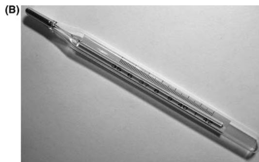
Figure 2 First thermometer—calibrated thermometer. The first calibrated thermometer (or thermometer) is credited to Sanctorio (1561–1636), who was driven to calibrate and measure all of the natural phenomena he observed. (A) is a wood cutting from the era, representing a stylistic depiction of the early Sanctorian thermometer. The hatch marks on the tube represent calibration lines. In (B) a modern-day mercury thermometer is shown.
