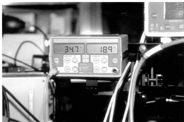
Figure 8 Two-channel electronic temperature monitor (Bi-Temp, Model TM-200D, Respiratory Support Products, Inc. SIMS, Irvine, California, U.S.A.). Core temperature is displayed on the left ( 34.7^{\circ}\text{C} ), and room temperature is displayed on the right ( 18.9^{\circ}\text{C} ). Low ambient operating room temperature, as seen in this example, is an important risk factor for intraoperative hypothermia in surgical patients.
