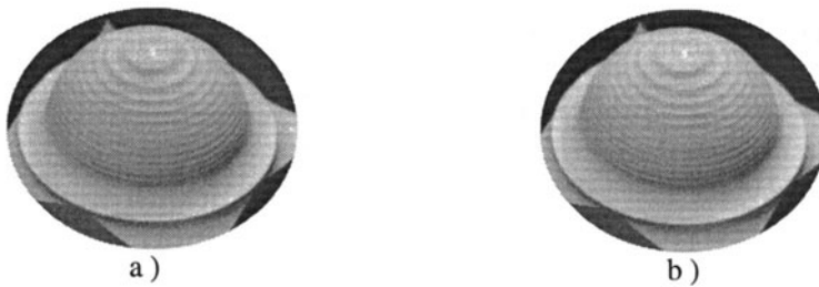
Figure 8: Semisphere \Phi_{0T}=40 mm. \xi_c=0.05 mm. a) Linear interpolation b) Reverse Bezièr
