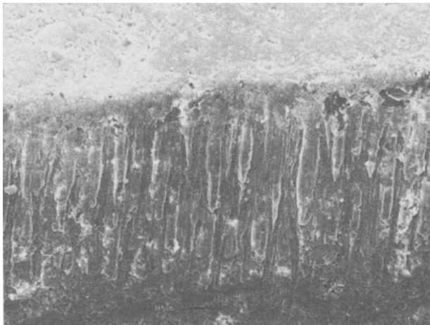
Fig. 2. Aspect of flank tool after testing at 7.8 m/s for 200 s. Alumina plastic deformation is evident.
