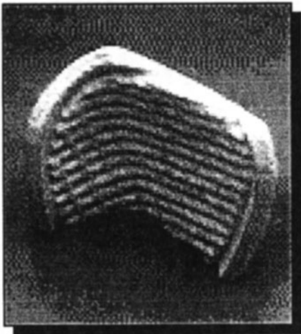
Fig. 8 – Door reflector (partial sector) prototype made with the STL file obtained from the CT stack of tomograms
