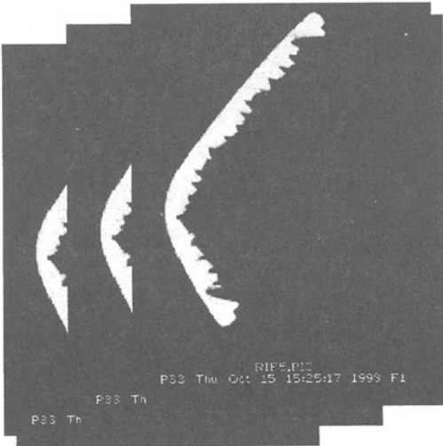
Fig. 2 – Three of the 80 tomograms included in the whole stack of CT acquisitions on the door reflector.
