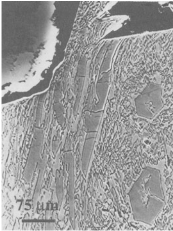
Fig 4a Cleavage cracks in the carbides
