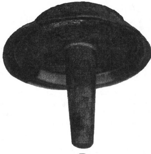
Fig.1 – The forged part after the blocking stage
