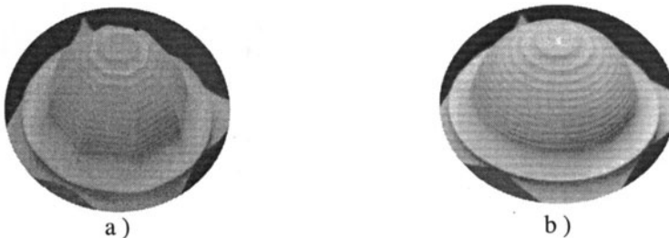
Figure 9: Semisphere \Phi_{0T}=40 mm. \xi_c=1 mm. a) Linear interpolation b) Intersection
