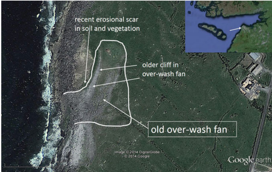
Fig. 5.16 Over-wash fan (with cobbles and small rounded boulders) from SSW behind the main boulder ridge, about 160 m long and eroded by two cliff-lines. The most recent cliff has been active again during the winter storms of 2013/14. Site is 5.9 km SW of Black Head, within Galway Bay (see insert) (Image credit ©Google earth 2014)
